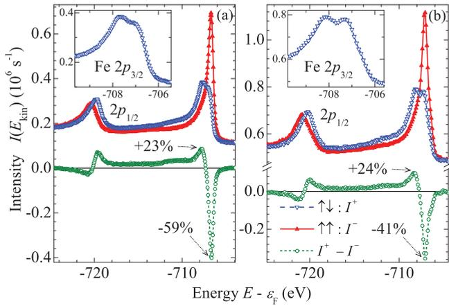
FIG. 8. (Color online) Polarization-dependent photoelectron spectra of the Fe  $2p$  core-level emission from CoFe on top of an IrMn exchange-biasing layer,  $\text{Co}_2\text{FeAl}$  beneath IrMn and the corresponding differences of the spectra taken with the opposite helicity of light. Asymmetry values are marked at selected energies. The insets show an enlarged view of  $I^+$  at the Fe  $2p_{3/2}$  states in both cases.
