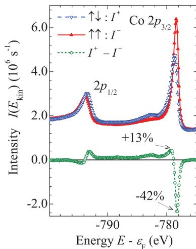
FIG. 4. (Color online) Polarization-dependent photoelectron spectra of the Co  $2p$  core-level emission from CoFe on top of an IrMn exchange-biasing layer and the difference of two spectra. Asymmetry values are marked at selected energies.
