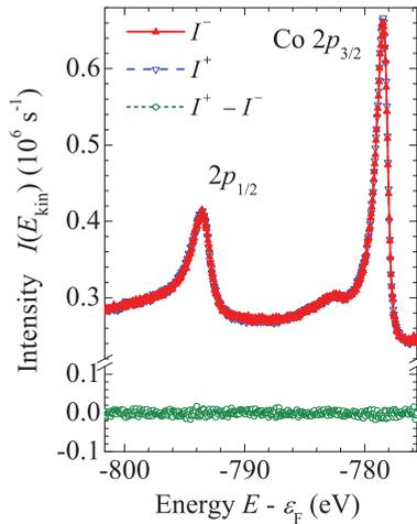
FIG. 5. (Color online) Illustration of the vanishing dichroism in photoemission when the photon polarization vector is perpendicular to the in-plane magnetization vector demonstrated for the Co  $2p$  state of CoFe. Shown are the photoelectron spectra  $I^+$ ,  $I^-$  and their difference  $I^+ - I^-$  obtained with different helicity at fixed magnetization perpendicular to the photon beam.
