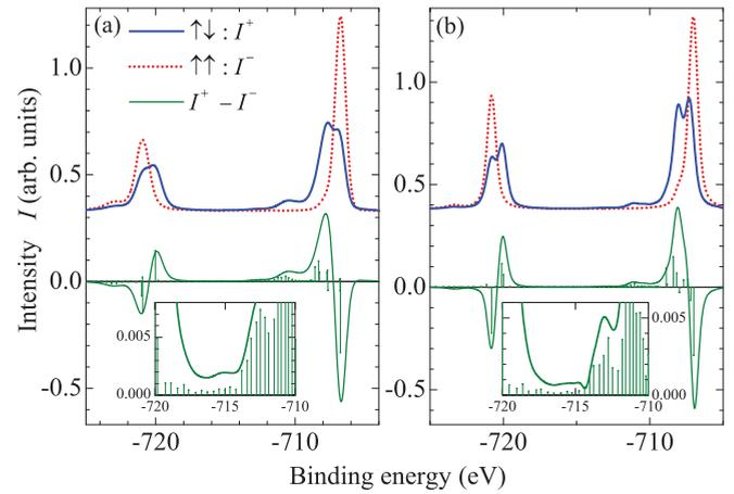
FIG. 9. (Color online) Calculated polarization-dependent photoelectron spectra of the Fe  $2p$  core-level emission obtained by means of atomic multiplet calculations and their difference for CoFe (a) and  $\text{Co}_2\text{FeAl}$  (b). The insets show the enlarged views of the difference curve in the region between spin-orbitally split components of Fe  $2p$  states. The bars mark the multiplet states.
