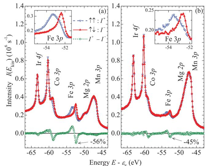
FIG. 7. (Color online) MCDAD for the shallow core level spectra obtained from the buried CoFe on top and  $\text{Co}_2\text{FeAl}$  beneath a 10-nm-thick IrMn film. The insets show an enlarged view of the Fe  $3p$  states.
