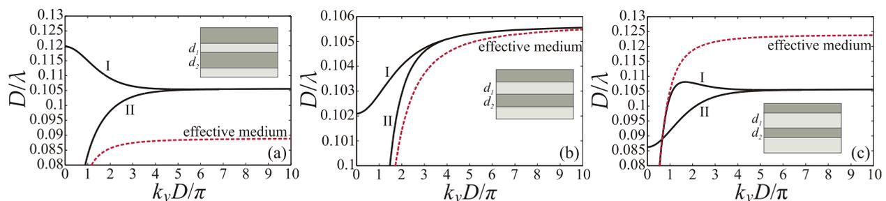
FIG. 2. (Color online) Dispersion diagrams and the geometries of the periodic nanostructures composed of alternating metal and dielectric layers. Thicknesses of the layers are (a)  $d_2 = 1.5d_1$ , (b)  $d_1 = d_2$ , and (c)  $d_1 = 1.5d_2$ . Two dispersion branches corresponding to the actual structures are numbered by Roman numerals.
