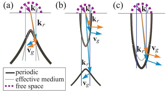
FIG. 3. (Color online) Diagrams of beam refraction at the air-MDN interface in the case of Fig. 2(c) at three different frequencies: (a)  $D/\lambda = 0.085$ , (b)  $D/\lambda = 0.094$ , and (c)  $D/\lambda = 0.106$ . Wave vectors  $\mathbf{k}_i$ ,  $\mathbf{k}_r$  of incident and refracted waves, respectively, and group velocity vectors  $\mathbf{v}_g$  are plotted by means of the isofrequency contours method. The first Brillouin zone is rendered.
