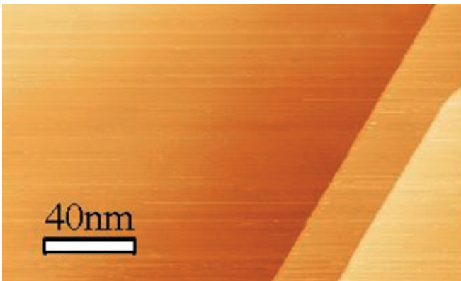
FIG. 1. (Color online) A scanning tunneling microscope (STM) image of a typically grown \text{Bi}_2\text{Se}_3 film with a thickness of 45 quintuple layers (QLs).
