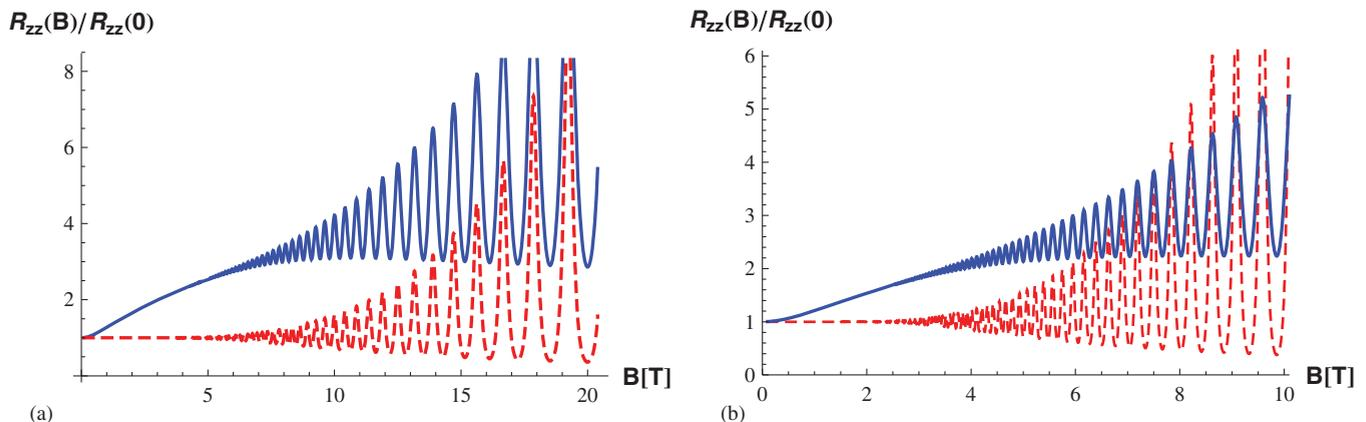
FIG. 1. (Color online) The MQO of resistivity  $R_{zz}(B) = 1/\sigma_{zz}$ , calculated using Eq. (34) with  $\Gamma_B$  given by Eq. (20) (solid blue line) and with  $\Gamma_B = \Gamma_0$ , which corresponds to Ref. 22 (dashed red line). The parameters used to plot (a) are  $m^* = 1.45m_e$ ,  $\Gamma_0 = 0.58$  K, and  $T = 1$  K. The parameters in (b) are  $m^* = m_e$ ,  $\Gamma_0 = 1$  K, and  $T = 0.6$  K.
