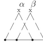
FIG. 4. The first diagram for the electron self-energy with the intersection of the impurity lines.
