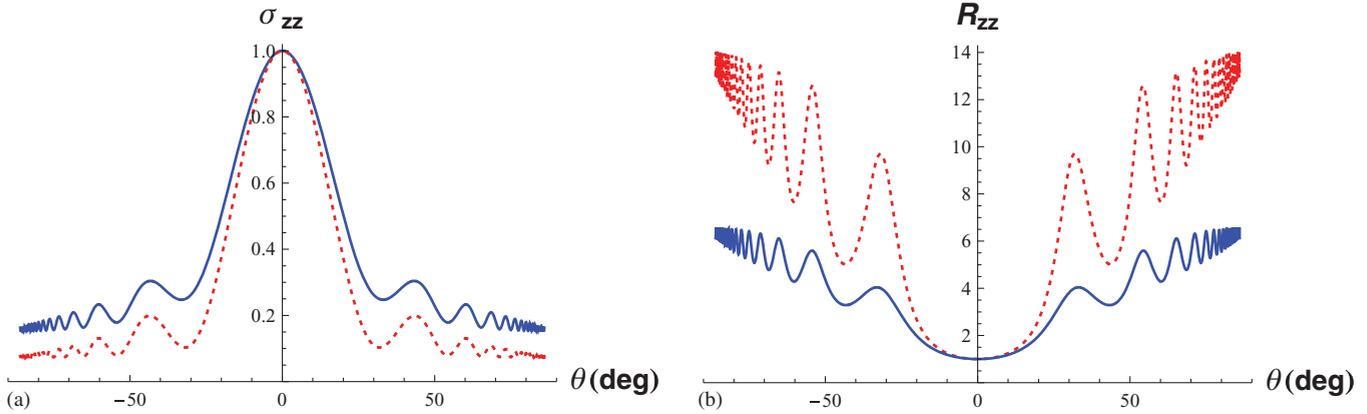
FIG. 2. (Color online) The angular dependence of conductivity  $\sigma_{zz}(\theta)/\sigma_{zz}(0)$  (a) and of magnetoresistance  $R_{zz}(\theta)/R_{zz}(0)$  (b), calculated using Eq. (36) with  $\tau_B$  given by Eq. (37) (solid blue line) and with  $\tau_B = \tau_0$  (dotted red line). The parameters for this plot are  $k_F d = 4$ ,  $m^* = m_e$ ,  $B = 3$  T,  $\Gamma_0 = 1$  K, which gives  $\omega_c \tau \approx 1.74$ .
