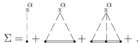
FIG. 5. The set of diagrams for the irreducible self-energy, corresponding to the self-consistent single-site approximation. The double solid line symbolizes the exact electron Green’s function.
