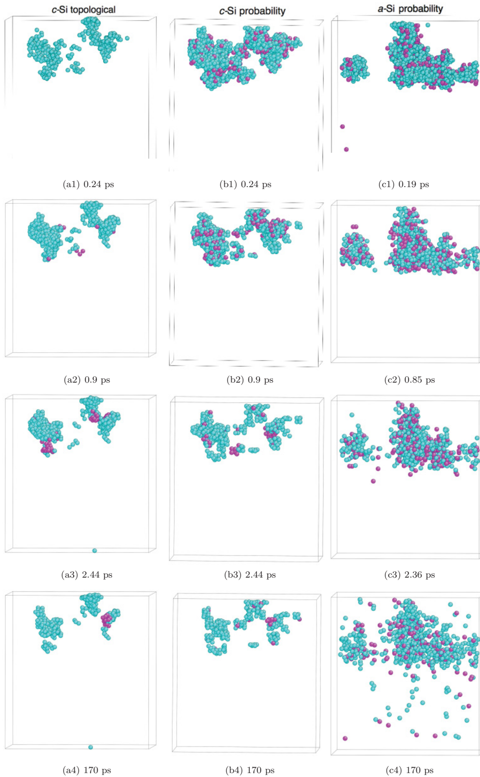
FIG. 1. (Color online) Distribution of defects in c -Si (left and center columns) and a -Si (right column) at times indicated. Only defective atoms are shown, as identified using the topological method (left column for c -Si) or the probability-function method (center column for c -Si, right column for a -Si). Atoms colored in purple (darker) are those that will return to a normal state within the following few time steps.
