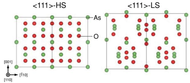
FIG. 4. (Color online) Projection of the  $\langle 111 \rangle$ -HS and -LS arrangements of  $As_2O_3$  from the  $[110]$  direction.
