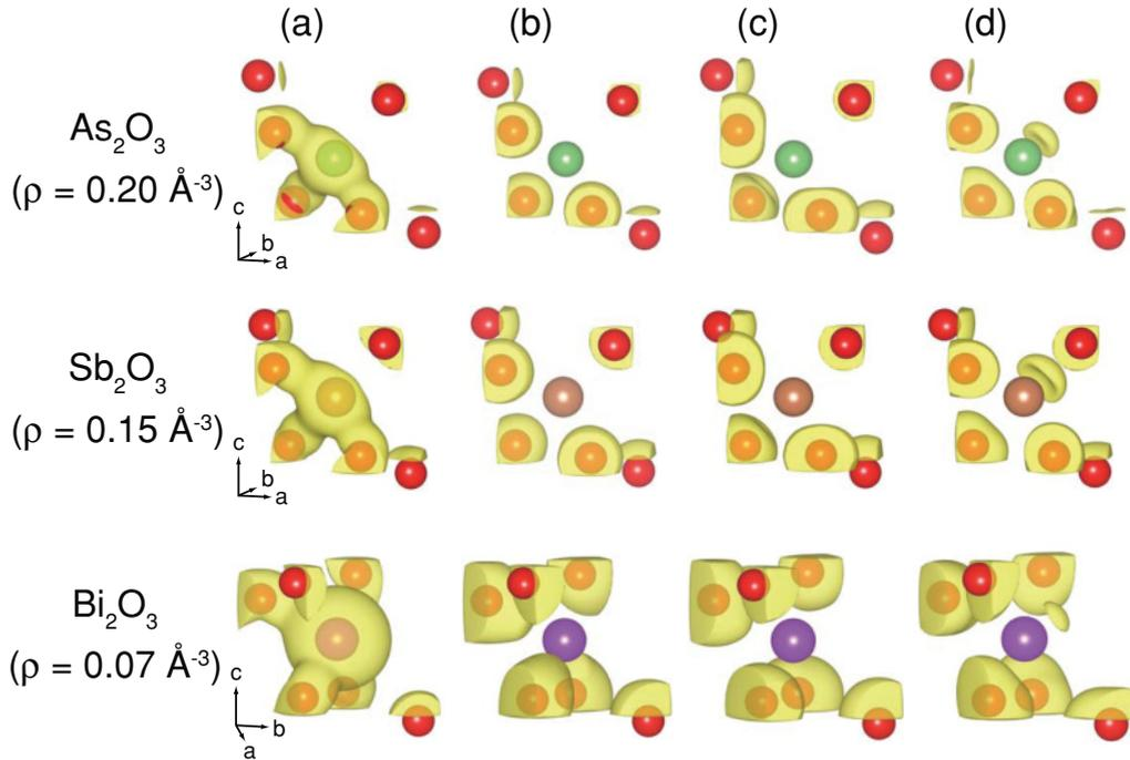
FIG. 9. (Color online) Isosurface of the valence electron density distribution in each region (see Fig. 8) around the cation in the  $\langle 111 \rangle$ -LS arrangement of the three sesquioxides. The isosurfaces of 0.20, 0.15, and  $0.07 \text{ \AA}^{-3}$  are shown for  $\text{As}_2\text{O}_3$ ,  $\text{Sb}_2\text{O}_3$ , and  $\text{Bi}_2\text{O}_3$ , respectively. Red spheres are oxygen ions. Green, brown, and violet spheres are cations.
