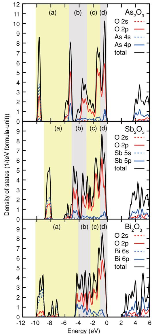
FIG. 8. (Color online) Partial electron density of states of the  $\langle 111 \rangle$ -LS arrangement for the three sesquioxides. The top of the valence band is set to 0. The black line represents the total density of states. Broken and solid red lines show the O 2s and O 2p states, respectively. Broken and solid blue lines represent the cation *ns* and *np* states, respectively. Four regions, (a)–(d), include the same number of valence electrons.
