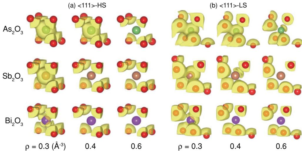
FIG. 7. (Color online) Isosurfaces of the valence electron density distribution around the cation in the (a)  $\langle 111 \rangle$ -HS and (b)  $\langle 111 \rangle$ -LS arrangements of the three sesquioxides. Part of the unit cell is extracted. Red spheres are oxygen ions. Green, brown, and violet spheres are cations.
