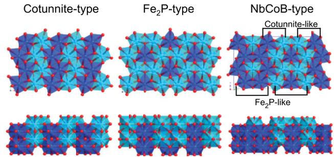
FIG. 2. (Color online) Crystal structures of  $\text{Fe}_2\text{P}$ -, cotunnite- and NbCoB-type phases. Blue and light blue spheres denote silicon atoms at different heights. Red small spheres denote oxygen atoms.
