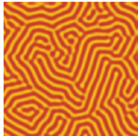
FIG. 6. (Color online) The u field for the case where \rho = 3.5 and \gamma = 0.12 (the point A in Fig. 3) at a scaled time of \tau = 1000 . The composition patterning observed is consistent with the prediction of linear theory.
