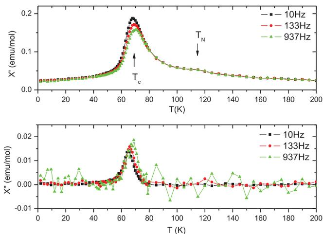
FIG. 11. (Color online) The real and imaginary components of  $\text{Co}_{2.25}\text{Fe}_{0.75}\text{O}_2\text{BO}_3$  magnetic susceptibility temperature dependences. The arrows indicate the magnetic transitions: a large peak near 70 K and a small anomaly near 115 K.
