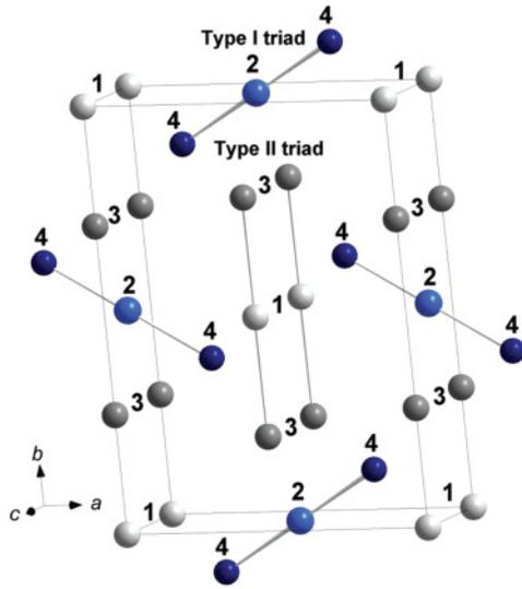
FIG. 1. (Color online) The crystal structure of  $M_2M'O_2BO_3$  ludwigites. The nonequivalent crystallographic sites 1, 2, 3, and 4 are numbered. The transition metal ions in the sites 2 and 4 form triads of type I, and the ions in the sites 1 and 3 form triads of type II.
