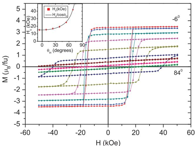
FIG. 6. (Color online) Hysteresis cycles of a  $\text{Co}_3\text{O}_2\text{BO}_3$  single crystal at  $T = 2$  K, as a function of rotation around the  $c$  axis. The extreme values of  $\theta_H$  are indicated. The inset shows the variation of  $H_c$  as a function of  $\theta_H$ . The fit to a  $1/\cos\theta_H$  function is also shown.
