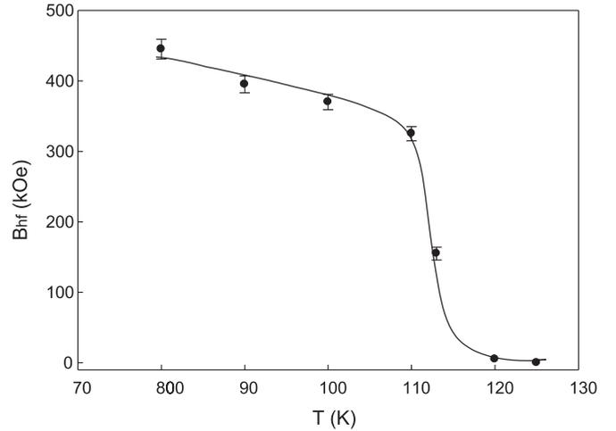
FIG. 4. The temperature dependence of the magnetic hyperfine field  $B_{hf}$  at iron ion nuclei at site 4 of  $\text{Co}_{2.25}\text{Fe}_{0.75}\text{O}_2\text{BO}_3$ . The solid line is a guide to the eye.
