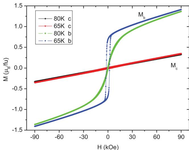
FIG. 14. (Color online) Hysteresis cycles as a function of  $T$  ( $T \geq T_N$ ).  $H$  applied along the  $b$  and  $c$  axes.
