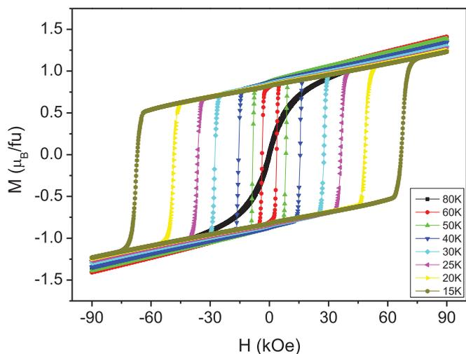
FIG. 15. (Color online) Hysteresis cycles of a  $\text{Co}_{2.25}\text{Fe}_{0.75}\text{O}_2\text{BO}_3$  sample as a function of  $T$  ( $T < T_N$ ).  $H$  parallel to the  $b$  axis.
