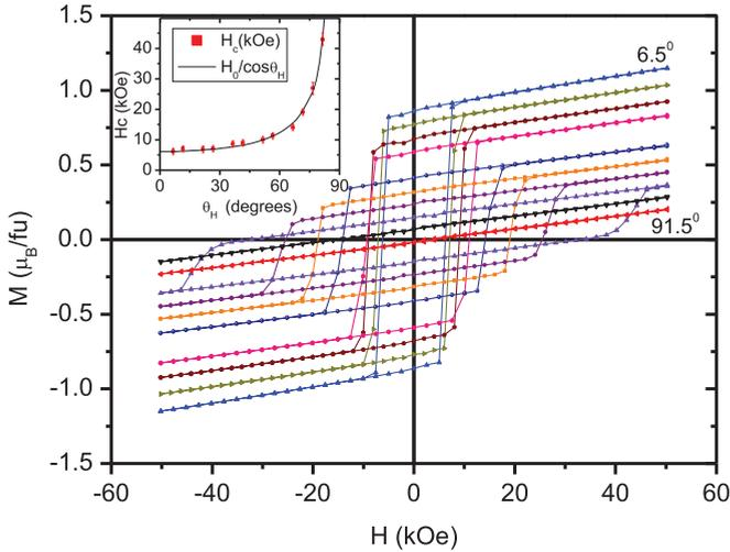
FIG. 17. (Color online) Hysteresis cycles of a  $\text{Co}_{2.25}\text{Fe}_{0.75}\text{O}_2\text{BO}_3$  single crystal at  $T = 50$  K, as a function of rotation around the  $c$  axis. The extreme values of  $\theta_H$  are indicated. The inset shows the variation of  $H_C$  as a function of  $\theta_H$ . The fit to a  $1/\cos\theta_H$  function is also shown.
