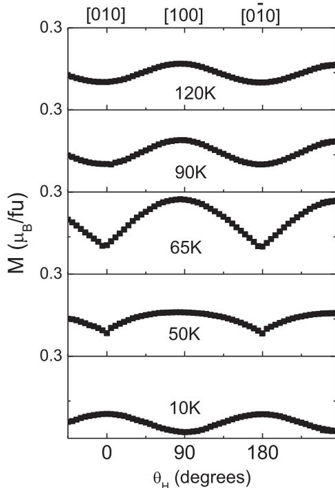
FIG. 7. The projection of the magnetization of  $\text{Fe}_3\text{O}_2\text{BO}_3$  in the direction of the applied field upon rotation around the  $c$  axis.  $H = 50$  kOe. Note the change of anisotropy EMD at  $10 \text{ K} < T_{N3}$  to the  $b$  axis, while at all other temperatures it is along the  $a$  axis.
