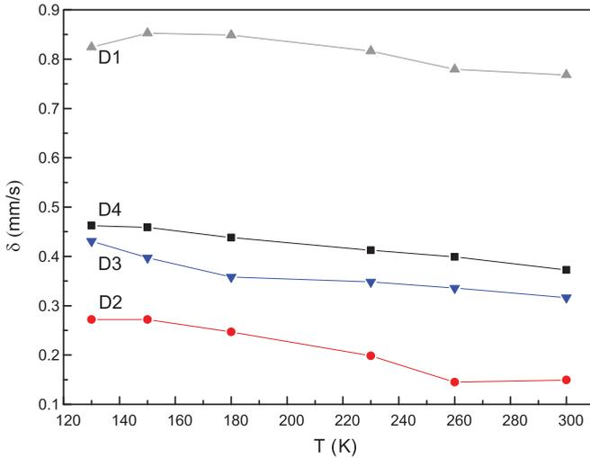
FIG. 3. (Color online) Temperature dependence of the isomer shift values obtained from the MS spectra for four quadrupole doublets (four nonequivalent iron sites) in the paramagnetic state of  $\text{Co}_{2.25}\text{Fe}_{0.75}\text{O}_2\text{BO}_3$ .
