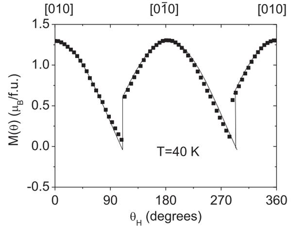
FIG. 13. The projection of the magnetization of  $\text{Co}_{2.25}\text{Fe}_{0.75}\text{O}_2\text{BO}_3$  in the direction of the applied field upon rotation around the  $c$  axis. Note the moment reversion at  $110^\circ$  and return at  $288^\circ$ .
