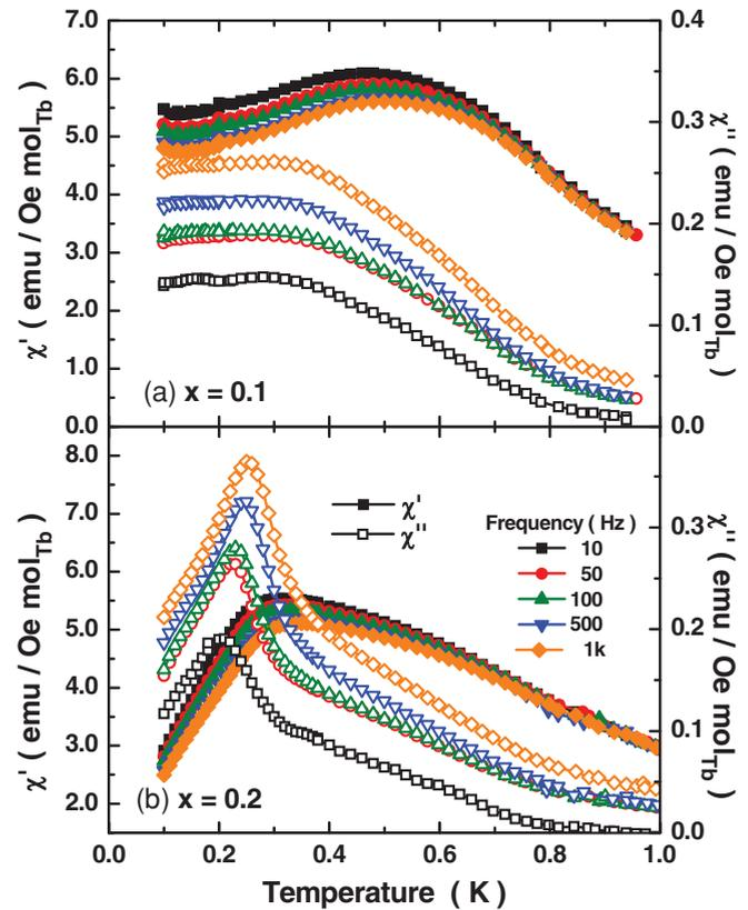
FIG. 5. (Color online) Frequency dependence of the  $x=0.1$  and  $x=0.2$  samples showing the suppression of ordering and the emergence of spin-glass-like behavior for  $x=0.2$ . Closed symbols show  $\chi'(T)$ ; open symbols show  $\chi''(T)$ .
