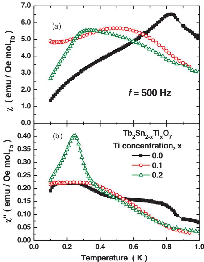
FIG. 4. (Color online) Dilution refrigeration ac magnetic susceptibility measurements on the three samples studied: the pure  $\text{Tb}_2\text{Sn}_2\text{O}_7$  and the two Ti-substituted samples in zero external applied field.
