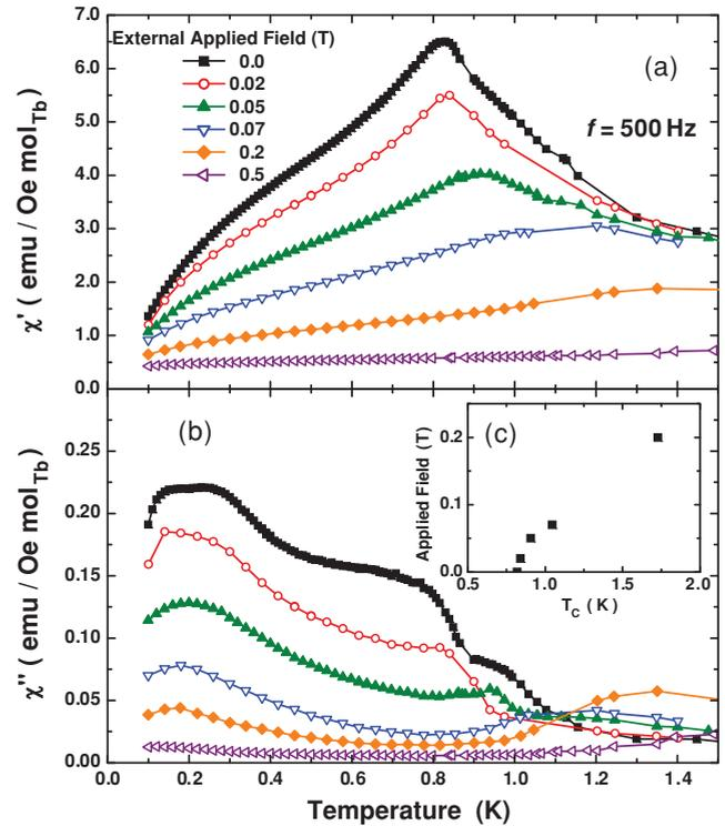
FIG. 3. (Color online) Low-temperature data taken on  $Tb_2Sn_2O_7$  in various external applied fields. (a)  $\chi'(T)$  clearly shows the ordering feature moving to higher temperature with increasing field as expected. (b)  $\chi''(T)$  shows the field dependence of the two low-temperature features. Inset (c) shows the dependence of the peak position on the external applied field.
