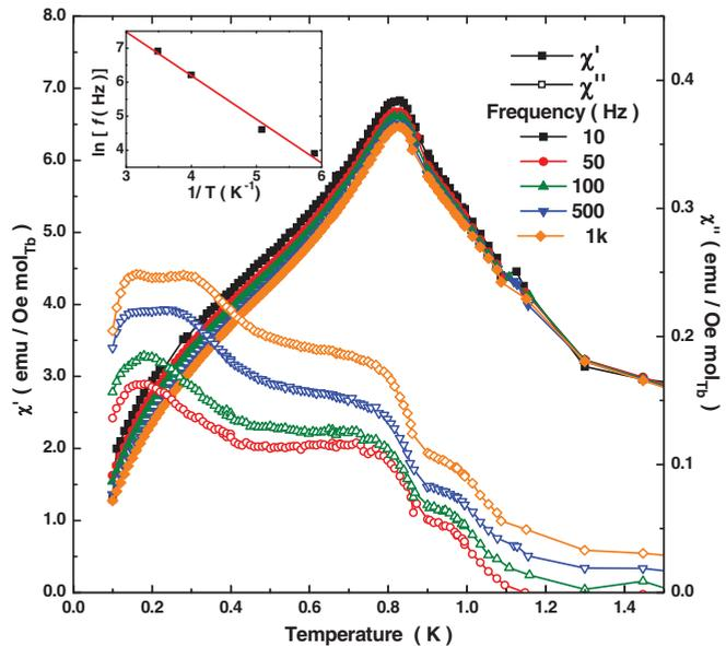
FIG. 2. (Color online) Low-temperature ac susceptibility of  $Tb_2Sn_2O_7$  in zero external applied field. Closed symbols show  $\chi'(T)$ ; open symbols show  $\chi''(T)$ . The inset shows an Arrhenius fit of the frequency dependence of the 300-mK feature.
