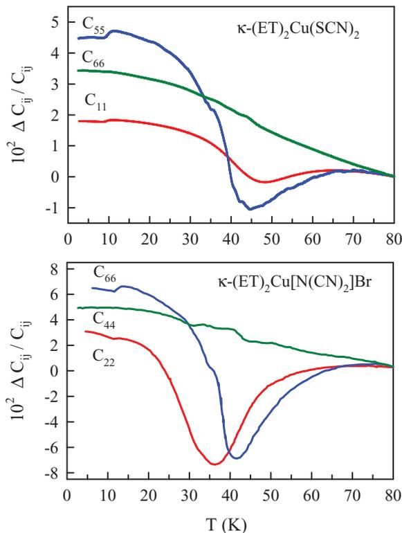
FIG. 1. (Color online) Temperature dependence of elastic moduli  $C_{ij}$  for two layered  $\kappa$ -(ET)<sub>2</sub>X organics.
