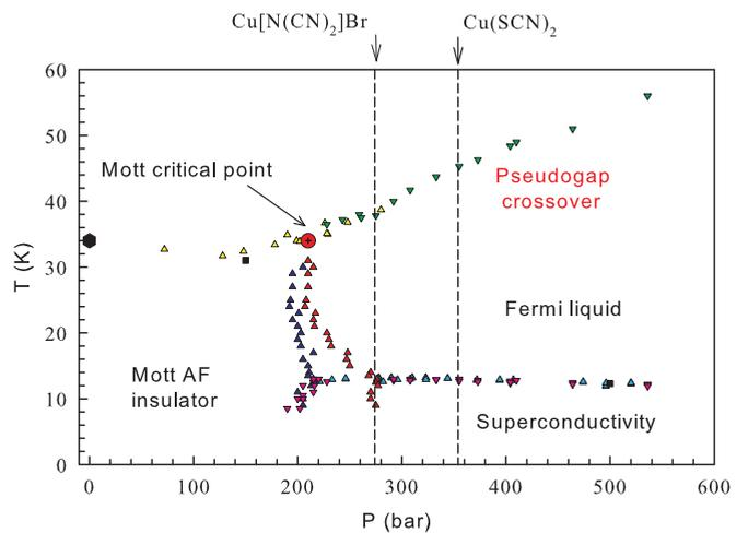
FIG. 2. (Color online) Temperature-pressure phase diagram of the layered  $\kappa$ -(ET)<sub>2</sub>Cu[N(CN)<sub>2</sub>]Cl organic compound taken from Ref. 14. The dashed lines indicate the position of the two compounds studied here,  $X = \text{Cu}(\text{SCN})_2$  and  $\text{Cu}[\text{N}(\text{CN})_2]\text{Br}$ , relative to the value of the pseudogap crossover temperature measured at ambient pressure.
