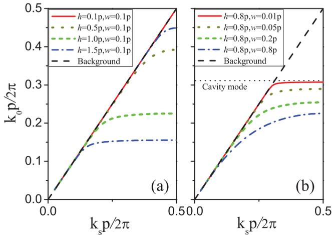
FIG. 1. (Color online) Dispersion curves for the systems made of rigid surfaces textured with a 1D periodical array of rectangular grooves, where  $p$ ,  $w$ , and  $h$  are the period, width, and depth of the grooves. The horizontal black dotted line in Fig. 1(b) denotes the frequency predicted by the first cavity mode for the given groove depth.
