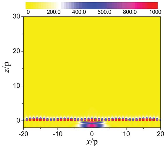
FIG. 4. (Color online) The numerical far-field distribution of the pressure amplitude (in arbitrary units) at the dimensionless frequency  $k_0 p/2\pi = 0.274$ .
