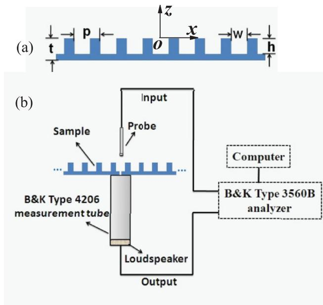
FIG. 2. (Color online) Schematic illustrations for (a) the sample consisting of an air-surrounded epoxy plate textured with a 1D periodical array of rectangular grooves along the  $x$  direction, with the geometric parameters given in the text, and (b) the experimental setup used for scanning the pressure field.
