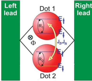
FIG. 1. (Color online) Model of our system showing two parallel quantum dots coupled to leads with spin exchange interaction between dots. A magnetic field in the region between dots provides a relative phase between electrons in the different dots as a result of the Aharonov-Bohm effect.
