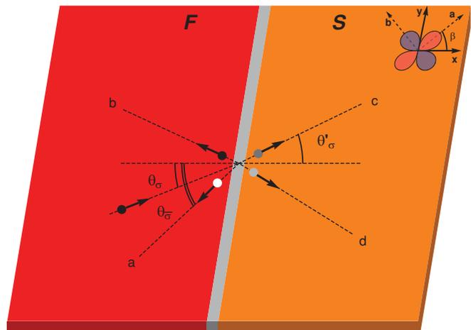
FIG. 1. (Color online) Scheme of the planar F/I/S junction analyzed in the paper. Here,  $\theta_\sigma$ ,  $\theta'_\sigma$ , and  $\theta''_\sigma$  are injection, Andreev reflection, and transmission angles, respectively, for electrons and quasiparticles with spin  $\sigma$ .  $\beta$  is the angle formed by the crystallographic *a* axis of a *d*-wave superconductor with the *x* axis.
