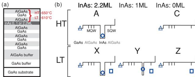
FIG. 1. (Color online) (a) Schematic description of the sample structure and (b) the corresponding conduction-band-minimum lineup. Upconversion centers of interest are indicated by circles, triangles, and squares (see text). In (b) the samples are grown from left to right. SQWs in samples A and C were grown at a high temperature (HT),  $\approx 650^\circ\text{C}$ ; samples X, Y, and Z, at a low temperature (LT),  $\approx 610^\circ\text{C}$ .
