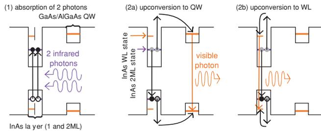
FIG. 5. (Color online) Sketch of the upconversion mechanism. (1) Two photons create two excitons in the 2-ML InAs island state. (2a) One exciton recombines and transfers its energy to the other exciton, whose electron and hole are excited and then relax to the GaAs/AlGaAs QW. (2b) Relaxation to the WL.
