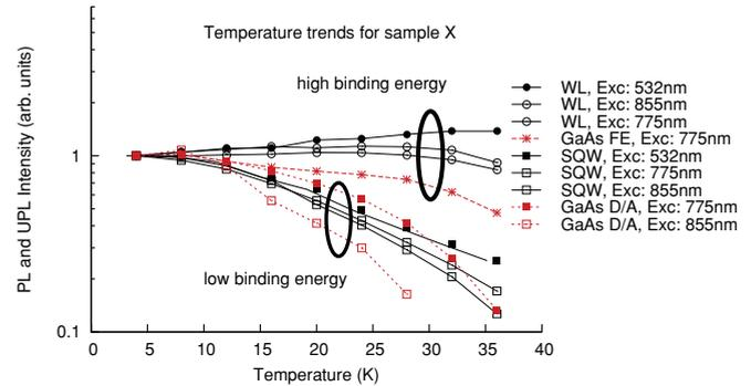
FIG. 4. (Color online) Temperature dependence of four PL peaks [SQW, WL, GaAs free exciton (FE), and GaAs donor/acceptor (D/A)] in Stokes (filled symbols) and anti-Stokes (open symbols) configurations, normalized by the 4 K data.
