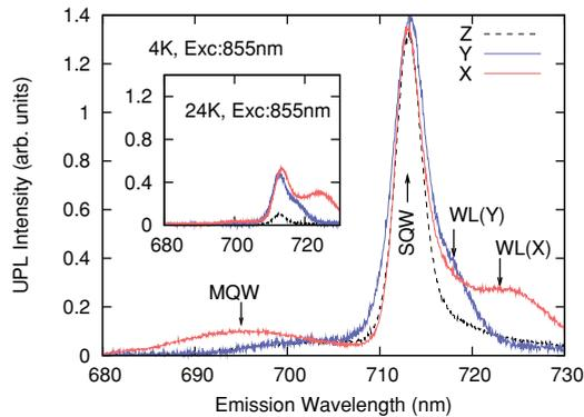
FIG. 3. (Color online) UPL spectra for samples X (2.2-ML InAs), Y (1.0-ML InAs), and Z (no InAs) excited at 855 nm, 10 W/cm<sup>2</sup>, measured at 4 K. Data are normalized to the deconvoluted SQW reference. Inset: data obtained at 24 K.
