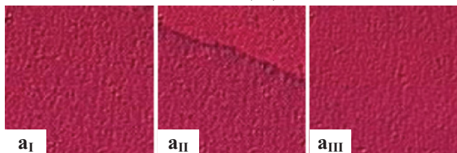
FIG. 6. (Color online) Zoom-in view of hysteresis loop along hard axis in TbFe/FeCo multilayer with 50 bilayers. (a I )–(a III ) are the micromagnetic images corresponding to the fields at three respective arrows marked in (a).
