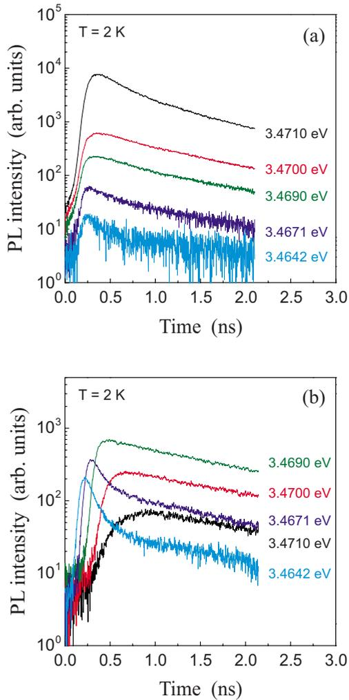
FIG. 9. (Color online) Decay curves for the emission just below NP DBE lines recorded in (a) conventional (reflection) mode and (b) transmission mode.
