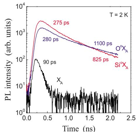
FIG. 3. (Color online) PL transients for the A free exciton and O and Si DBE no-phonon lines at 2 K.
