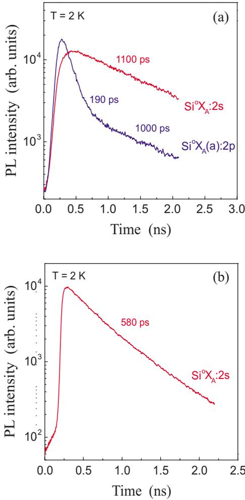
FIG. 7. (Color online) (a) PL transients of the 2s and 2p TETs related to the Si donor. (b) PL transient of the 2s TET related to the Si donor in sample no. 1. The shorter decay time in comparison with the sample no. 2 is presumably due to the larger background doping concentration.
