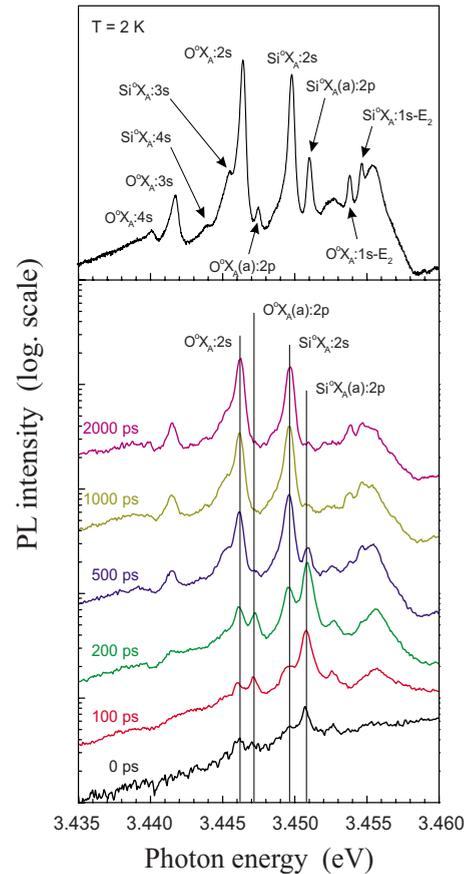
FIG. 6. (Color online) Time-resolved PL spectra at 2 K in the energy region of the two-electron transitions. All spectra are normalized and vertically shifted for clarity. The vertical lines mark the most intense emission lines for which PL transients are extracted. At the top continuous-wave PL spectrum is shown. The TETs are labeled with the initial state DBE (shown only for excited states) and the final state of the donor (1s, 2s, 2p, etc.).
