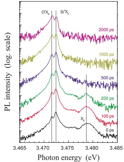
FIG. 2. (Color online) Time-resolved PL spectra at 2 K for sample no. 2 in the energy region of the no-phonon DBE emission lines. The spectra are normalized and vertically shifted for clarity. The vertical lines mark the emission lines for which PL transients are shown in Fig. 3.
