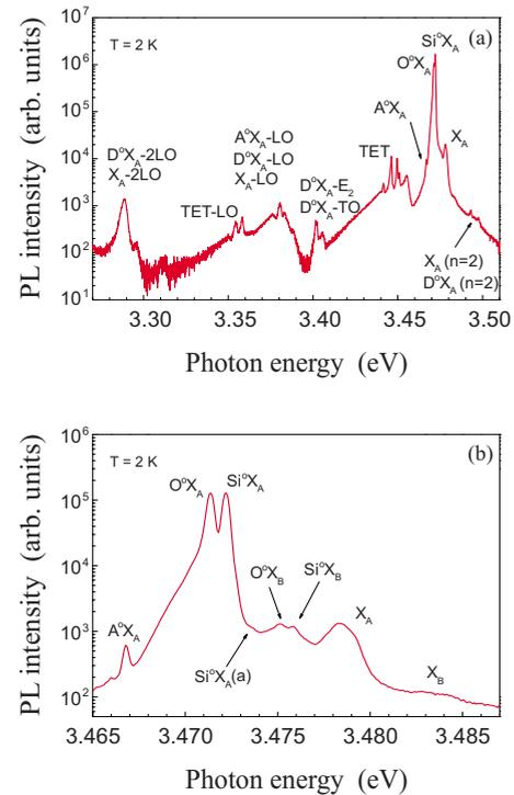
FIG. 1. (Color online) (a) Near band-gap PL spectrum at  $T=2$  K for sample no. 2. The spectrum shows the FE and BE no-phonon lines, the two electron transition lines, and the corresponding phonon replicas. (b) High-resolution spectrum in the region of the no-phonon exciton lines. The excited states of DBEs are labeled (a), (b), etc.
