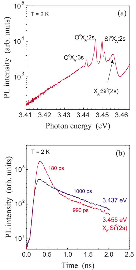
FIG. 8. (Color online) (a) Enlarged PL spectrum in the energy range of TETs showing the broad continuum background. (b) PL transients for the emission at 3.455 eV (recombination of A exciton scattered by Si donors) and 3.437 eV (continuum of TETs).
