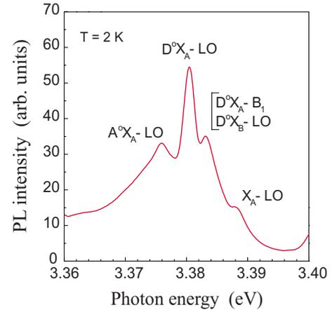
FIG. 4. (Color online) Low-temperature PL spectrum (2 K) in the region of the first LO-phonon replicas of free and bound excitons.
