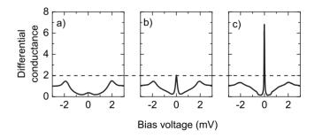
FIG. 3. Evolution of the zero-bias peak with increasing contact size at T=1.6 K. Dashed lines indicate the upper theoretical limit for the peak amplitude in NS junctions,  $G_{max}(V=0)=2 \cdot G_{normal}$ . The differential conductance curves are normalized to the normal state resistances of the contacts, which are: (a) 994  $\Omega$ , (b) 250  $\Omega$ , and (c) 130  $\Omega$ , respectively.
