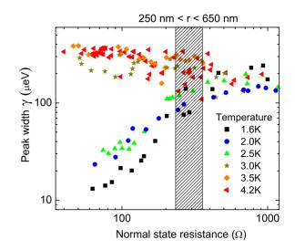
FIG. 2. (Color online) Width of the zero-bias peak as a function of contact resistance at different temperatures. Dashed area shows the transition region in the contact resistance and the corresponding contact diameter.
