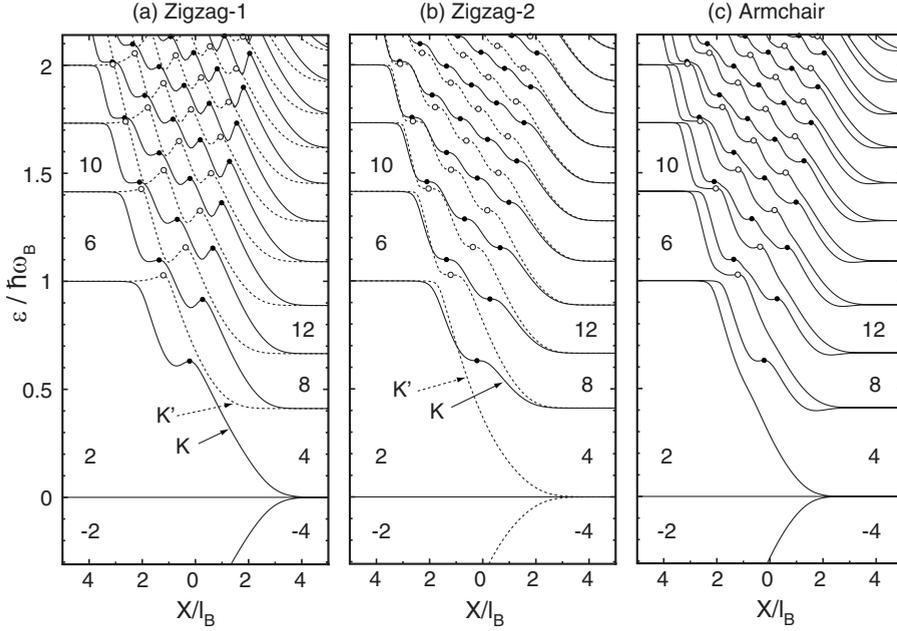
FIG. 3. Energy spectrum as a function of  $X$  in boundary (a) ZZ1, (b) ZZ2, and (c) AC at magnetic field  $\hbar\omega_B = \gamma_1/3$  ( $B \sim 13$  T). Black and white circles represent  $P_K$  and  $P_{K'}$ , respectively. Numbers between the levels indicate bulk filling factor in limits  $X = \pm\infty$ .
