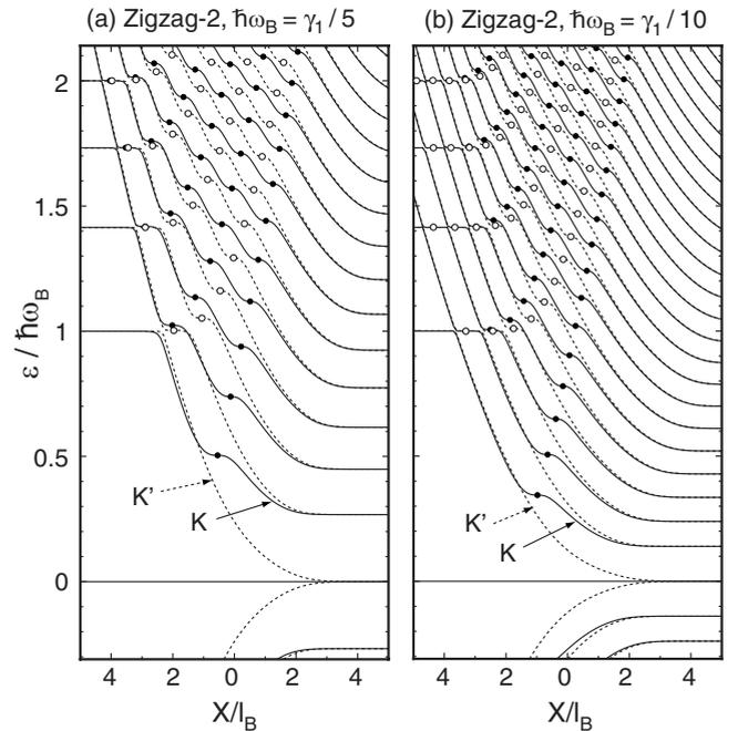
FIG. 4. Energy spectrum as a function of  $X$  in boundary ZZ2 at magnetic fields (a)  $\hbar\omega_B = \gamma_1/5$  ( $B \sim 5$  T) and (b)  $\gamma_1/10$  ( $B \sim 1.2$  T).
