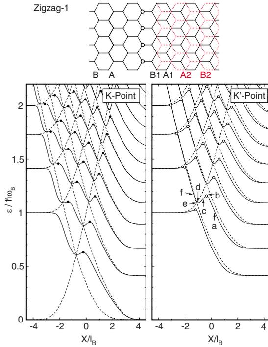
FIG. 5. (Color online) (Above) Monolayer-bilayer junction of type ZZ1, separated by infinite potential on white circles into independent monolayer and bilayer graphenes. (Below) Energy spectrum of junction ZZ1 (solid) and separated system (dashed) in magnetic field  $\hbar\omega_B = \gamma_1/3$ . Left and right panels show the spectra of the  $K$  and  $K'$  points, respectively, and the black and white circles are the interface Landau levels.
