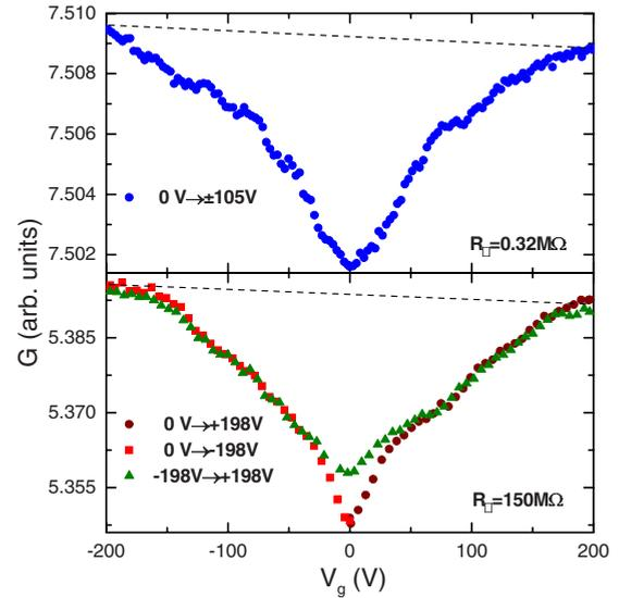
FIG. 5. (Color online) The conductance versus gate voltage for two Be films (labeled by their  $R_{\square}$  illustrating the memory-dip structure. After the sample was allowed to equilibrate under  $V_g = 0$  for  $\approx 24$  h, scans were taken either from  $V_g = 0$  in each voltage direction [symmetrical  $G(V_g)$  scans] or, from  $-198$  to  $+198 V$ . Note that the structure is skewed due to the contribution of the antisymmetric (equilibrium) field effect (see text).
