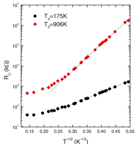
FIG. 1. (Color online) Resistance versus temperature plots for two of the beryllium films used in this study.
