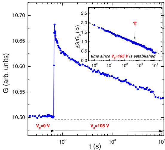
FIG. 4. (Color online) A gate-excitation protocol for a specific Be sample ( $R_{\square} = 40 M\Omega$ ). The inset depicts the characteristic  $\log(t)$  dependence of the EG from which the typical relaxation time  $\tau$  is estimated using the baseline conductance  $G_0$  ( $105 V$ ) (marked here by the dashed line) measured independently.
