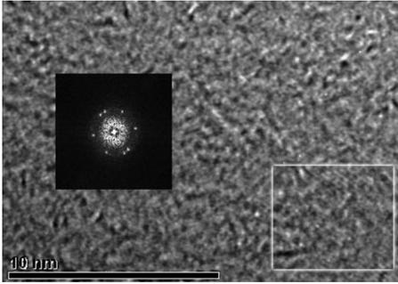
FIG. 2. Transmission electron microscope micrograph of  $\approx 20$  Å Be film deposited on carbon-coated Cu grid. The black square is a Fourier transform of the framed area on the right. The latter shows 2.33 Å fringes associated with the  $d$  spacing of the  $\langle 100 \rangle$  planes of the hexagonal BeO (reflected as satellites in the Fourier transform plate).
