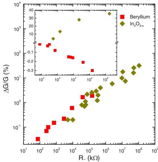
FIG. 6. (Color online) The relative magnitude of the memory dip versus  $R_{\square}$  for the studied Be samples. The data of Ref. 15 are shown for comparison. Insert: The slope (relative change in  $G$  per 400 V of  $V_g$ ) of the antisymmetric part of  $G(V_g)$  compared with typical results for  $\text{In}_2\text{O}_{3-x}$  samples.
