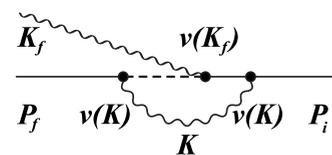
FIG. 3. Vertex correction to single phonon scattering in third-order perturbation theory.
