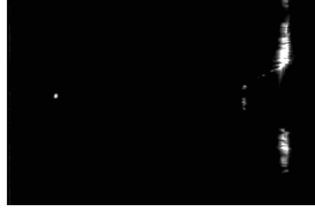
FIG. 7. Photo of the trap with a confined visible graphene flake. The particle is on the left while scattering from the faces of the electrodes is visible on the right.
