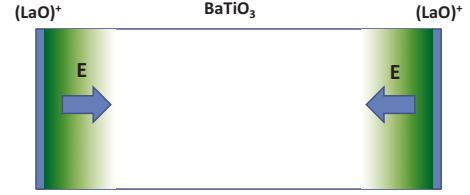
FIG. 1. (Color online) Charge distribution and the intrinsic electric field in a BaTiO 3 film terminated with positively charged (\text{LaO})^+ monolayers at the left and right interfaces. A gradient shadow region indicates the screening charge penetrating into BaTiO 3 . Arrows indicate the intrinsic electric field that has a tendency to pin the local polarization along the field direction.
