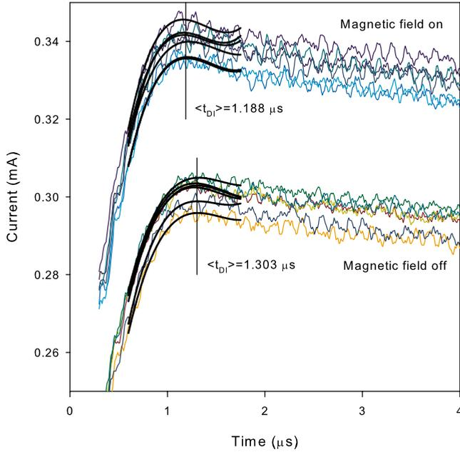
FIG. 4. (Color online) A set of DI curves and fits for the ambipolar device with an offset voltage above turn on (3.5 V) both with and without a magnetic field to show that the effect of the  $B$  field can be reliably measured.
