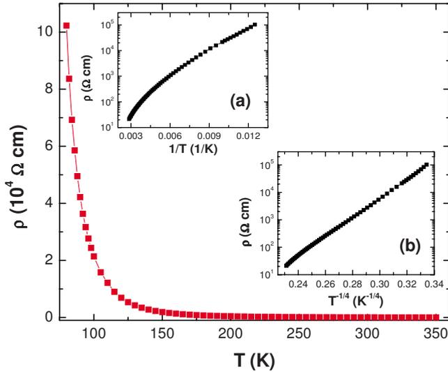
FIG. 3. (Color online) The in-plane electrical resistivity  $\rho$  versus temperatures  $T$  for a single crystal of  $\text{Na}_2\text{IrO}_3$ . The inset (a) shows the  $\rho$  versus  $1/T$  data on a semi-log scale. The inset (b) shows the  $\rho$  versus  $1/T^{1/4}$  data on a semi-log scale.
