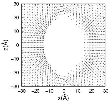
FIG. 2. Current-density  $\mathbf{j}(\mathbf{r})=\rho(\mathbf{r})\mathbf{v}(\mathbf{r})$  map for the same configuration shown in Fig. 1. The length of the arrows is proportional to the value of  $|\mathbf{j}|$ . The maximum value shown in the figure corresponds to the peak in the following Fig. 3.
