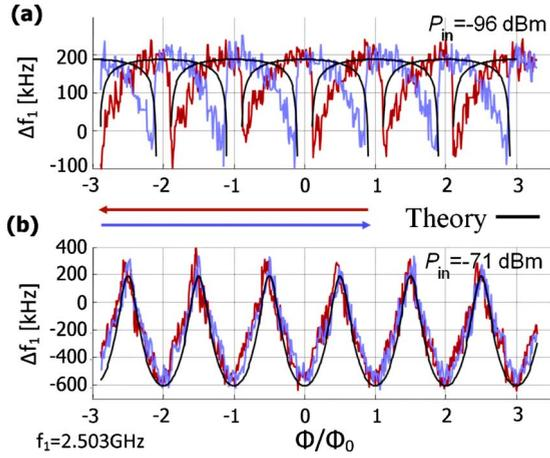
FIG. 3. (Color online) The resonance frequency shift  $\Delta f_1$  of the first (detector) mode vs. applied flux for two different values of  $P_{in}$ . The flux is first swept upwards (blue line) and then downwards (red line). The black solid lines represent the theoretical calculation of  $\Delta f_1$  using the following parameters:  $\beta_L=7.4$  for  $P_{in}=-96$  dBm,  $\beta_L=0.15$  for  $P_{in}=-71$  dBm, and  $I_{c1}/I_{c2}=3$  for both cases.
