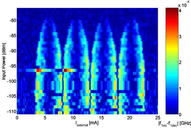
FIG. 7. (Color online) The difference between the measured resonance frequencies obtained in the increasing flux sweep ( $f_{1 \text{ inc}}$ ) and the decreasing flux sweep ( $f_{1 \text{ dec}}$ ) of the first (*detector*) mode. The dark blue areas correspond to monostable regions, namely, the same resonance frequency is measured for both the increased and decreased sweep. The red indicates the regions where the system is bistable.
