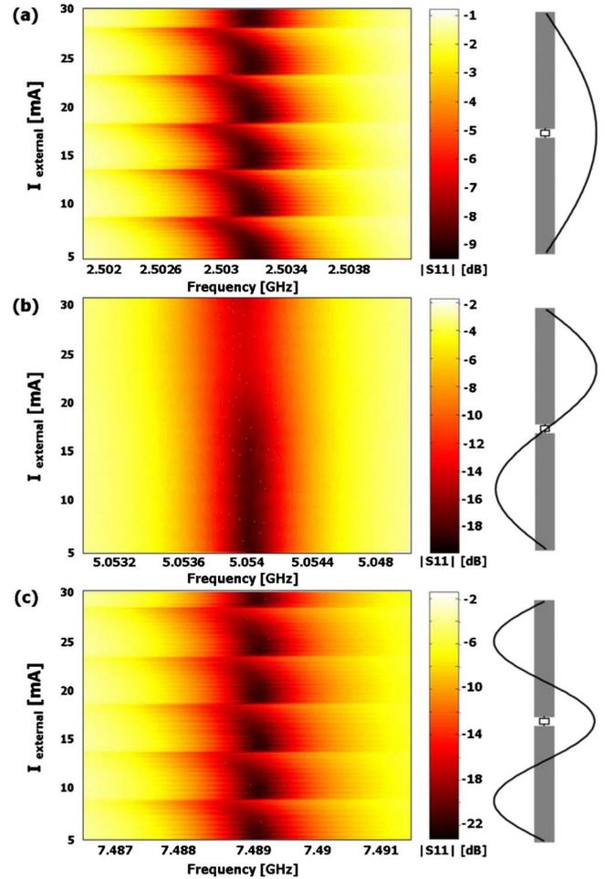
FIG. 2. (Color online) Reflection coefficient  $|S_{11}|$  vs frequency and external flux for the first 3 modes of the SSR. A change of 4.8 mA in the external current corresponds to a change of  $\Phi_0$  in the magnetic flux.
