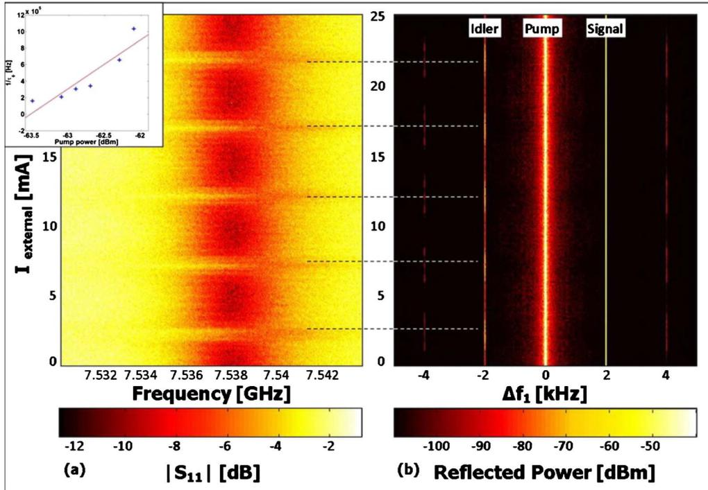
FIG. 4. (Color online) IM characterization of the detector mode [panel (b)] and  $|S_{11}|$  measurements of the system mode [panel (a)]. Largest idler gain as well as highest dephasing rate is obtained at half integer values of the externally applied flux. The pump frequency is  $\omega_p=\omega_1(\Phi=0)$ . The inset shows the dephasing rate as a function of the pump power.
