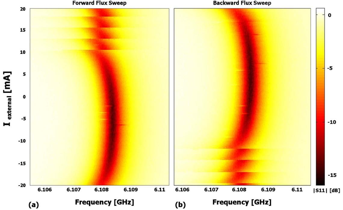
FIG. 6. (Color online) Measured  $|S_{11}|$  at input power  $P_{in} = -95$  dBm for (a) forward and (b) backward magnetic flux sweep. In this sample  $\beta_L = 20$ , and the response is highly hysteretic.
