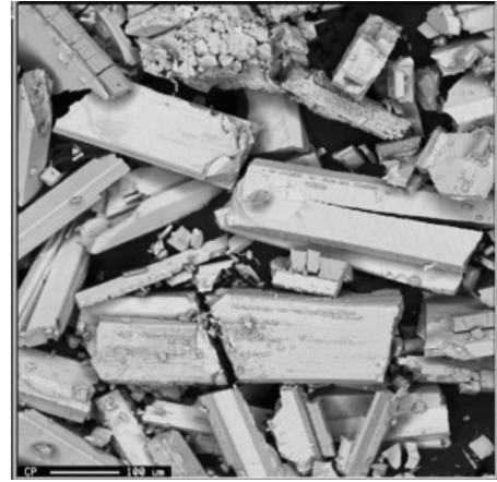
FIG. 3. Photo of cobalt-antimonium hulsite-type crystals using backscattered electron imaging in WDS measurements.
