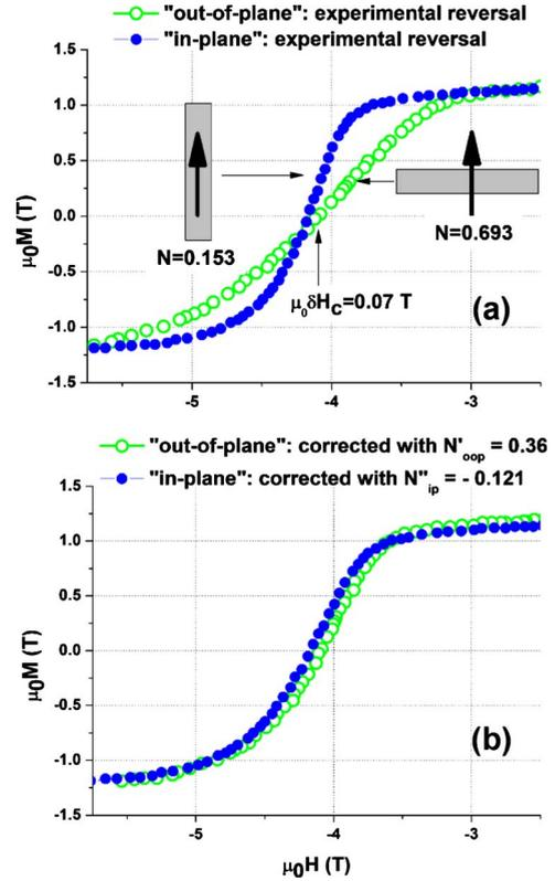
FIG. 5. (Color online) (a) Experimental magnetization curves of NdFeB platelets with “oop” (having  $N = 0.693$ ) and “ip” ( $N = 0.153$ ) geometries. (b) Applying the general Hard-Demag corrections  $N''$  ( $N'' \equiv N''$  for the oop case) yields two parallel curves, thus revealing the applicability of the model.
