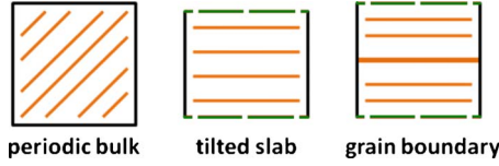
FIG. 2. (Color online) The three systems considered in excess potential energy calculations. Orange lines are Miller planes; green dashed lines are fixed free surfaces.
