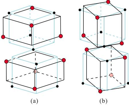
FIG. 7. (Color online)  $\mathbf{q}=0$  lattice phonons with (a)  $E_g$  and (b)  $F_{1g}$  symmetries in a spinel structure. These normal modes are dominated by oxygen displacements. The red and black circles indicate oxygen and vanadium ions, respectively.
