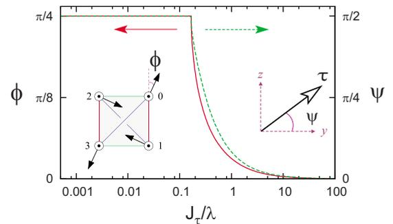
FIG. 6. (Color online) Evolution of orthogonal magnetic order as a function of the ratio  $J_\tau/\pi$ . The parameter  $\psi$  and  $\phi$  measure the rotation angle of pseudospin and in-plane orthogonal structure, respectively. The SO coupling constant is set to  $\lambda = 0.75\Delta$  and the ferromagnetic spin component is  $S_z = 1/\sqrt{3}$ . The limiting cases  $\phi = \pi/4$  and  $0$  correspond to magnetic orders shown in Figs. 5(b) and 5(d), respectively.
