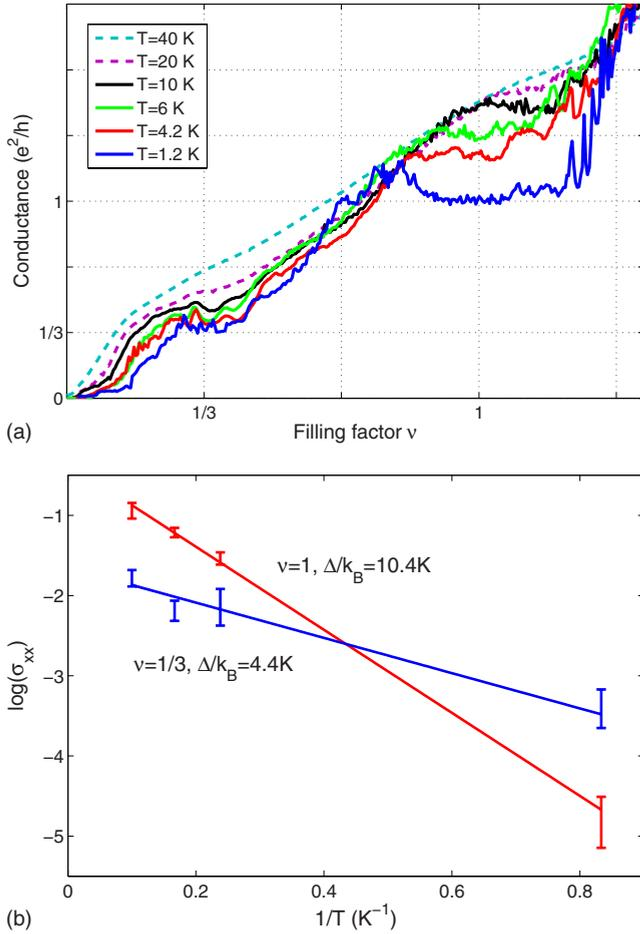
FIG. 3. (Color online) (a) Temperature dependence of the two-terminal conductance from which  $\sigma_{xx}$  on the  $\nu=1/3$  and  $\nu=1$  plateaus is extracted. (b) Fits of the temperature dependence of  $\sigma_{xx}$  to the activation model,  $\sigma_{xx} \sim \exp(-\Delta/2k_B T)$ . The best-fit values of the activation gap are  $\Delta_{\nu=1}=10.4$  K and  $\Delta_{\nu=1/3}=4.4$  K. The procedure used to estimate error bars is outlined in Fig. 2.
