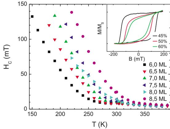
FIG. 4. (Color online) Temperature-dependent coercivities of series (A) samples with  $x=50$  at. % Fe. Inset: Fe-concentration-dependent hysteresis curves of the same three 15 ML Ni/6.5 ML  $\text{Fe}_x\text{Mn}_{1-x}/\text{Cu}(001)$  samples as in Fig. 1 measured at 190 K.
