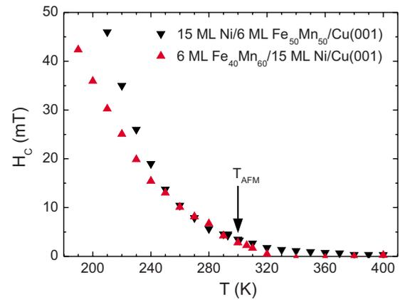
FIG. 3. (Color online) Temperature-dependent coercivities of two samples [series (B)] with the same  $Fe_xMn_{1-x}$  layer thickness but opposite layer sequence.
