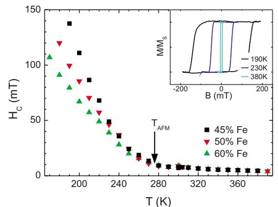
FIG. 1. (Color online) Temperature-dependent coercivities obtained from hysteresis curves of 15 ML Ni on 6.5 ML Fe<sub>x</sub>Mn<sub>1-x</sub> for different Fe concentration [series (A)]. The inset shows examples of normalized polar MOKE hysteresis curves of the Fe<sub>45</sub>Mn<sub>55</sub> sample at different temperatures.
