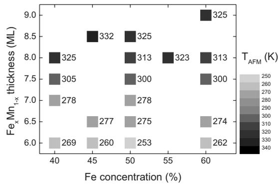
FIG. 2. Grayscale-coded AFM ordering temperature ( $T_{AFM}$ ) of all samples from series (A) in dependence of the  $Fe_xMn_{1-x}$  thickness and Fe concentration. Numbers denote  $T_{AFM}$  in Kelvin ( $\pm 5$  K).
