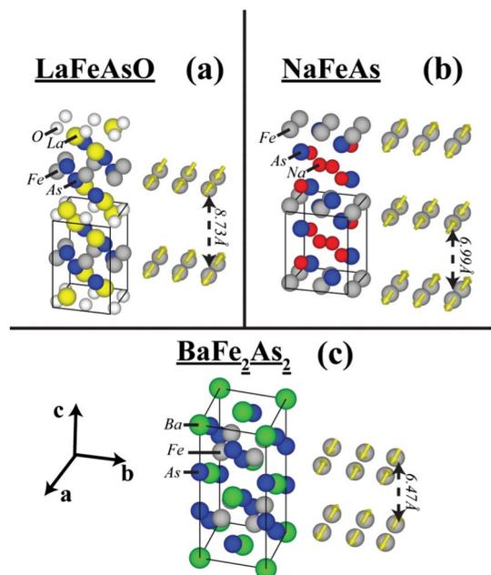
FIG. 1. (Color online) Crystal structures of representative materials from the (a)  $REFeAsO$ , (b)  $AMFeAs$ , and (c)  $AFe_2As_2$  classes of iron arsenides. Boxes show the enclosed chemical unit cells of each system. To the right of each chemical structure are plotted the ordered spin systems. Moment directions are plotted as yellow arrows located on the Fe sites.
