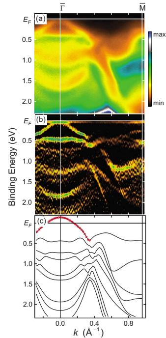
FIG. 2. (Color online). (a) Photoemission results from a 6 BL Bi film in the PC phase. (b) Second derivative along the energy axis of the photoemission data to enhance the contrast. (c) Calculated band structure. The top band, marked by small circles, has a surface character.
