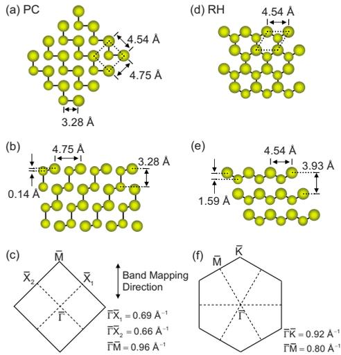
FIG. 1. (Color online). (a) Top view of (110), (b) side view along  $[1\bar{1}0]$ , and (c) surface Brillouin zone of the PC structure. (d) Top view of (111), (e) side view along  $[11\bar{2}]$ , and (f) surface Brillouin zone of the RH structure. Larger balls indicate atoms closer to the viewer. The direction of photoemission band mapping is indicated.
