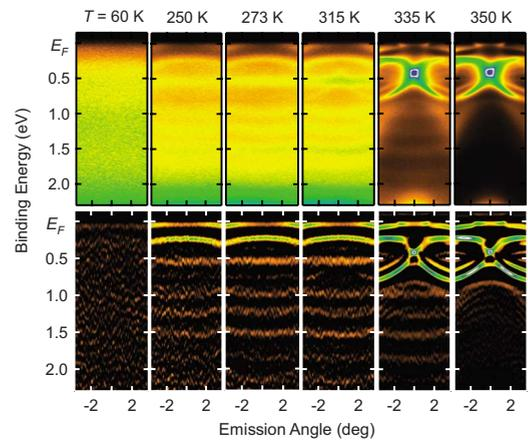
FIG. 5. (Color online). Top row: Photoemission results from a Bi film of thickness 14 BL (referred to the RH structure) after annealing to various temperatures as indicated. The structure of the film changes from a disordered phase to the PC phase first, then to a mixed phase, and finally to the RH phase. Bottom row: Second derivative of the same data.
