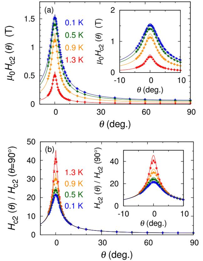
FIG. 4. (Color online) (a) Field-angle  $\theta$  dependence of the upper critical field  $H_{c2}$  of  $\text{Sr}_2\text{RuO}_4$  at various temperatures for  $\phi=0^\circ$ . (b) Angle  $\theta$  dependence of  $H_{c2}$  normalized by  $H_{c2}(\theta=90^\circ)$ . Solid curves are the fitting results using Eq. (3) in the range  $2.5^\circ \leq |\theta| \leq 90^\circ$ . Insets are enlarged views near  $\theta=0^\circ$ .
