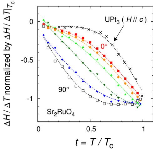
FIG. 3. (Color online) Temperature dependence of the slope of the  $H$ - $T$  phase diagram of  $\text{Sr}_2\text{RuO}_4$  at  $\theta=90, 5, 2, 1, 0.5$ , and  $0^\circ$  from bottom to top for  $\phi=0^\circ$ . The slope of the  $H_{c2}$  curve for  $\text{UPT}_3$  (Ref. 18), evaluated from the dashed curve in the inset of Fig. 2(b), is also plotted with crosses. The dashed curves are guides to the eyes.
