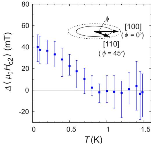
FIG. 7. (Color online) Temperature dependence of the in-plane  $H_{c2}$  anisotropy between  $\phi=0^\circ$  and  $\phi=45^\circ$  at  $\theta=0^\circ$ .  $\Delta(\mu_0 H_{c2})$  is defined as  $\mu_0 H_{c2}(\phi=45^\circ) - \mu_0 H_{c2}(\phi=0^\circ)$ .
