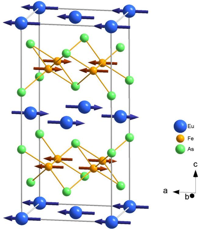
FIG. 6. (Color online) Illustration of the magnetic structures of  $\text{EuFe}_2\text{As}_2$  at 2.5 K. The Fe moments align along  $a$  direction and order antiferromagnetically in both  $a$  and  $c$  directions. The Eu moments align along  $a$  direction and order antiferromagnetically in  $c$  direction only. The gray line outlines the orthorhombic unit cell.
