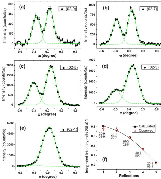
FIG. 4. (Color online) (a)–(e) Omega scans of series of  $(02l)$  (with  $l = \text{odd}$ ) reflections at 2.5 K. The integrated intensities of  $(20l)$  and  $(02l)$  can be obtained by fitting the curves with two Gaussian functions. (f) The ratio between  $(20l)$  and  $(02l)$  reflections shows good agreement with the calculated value.
