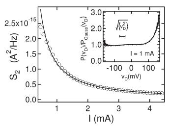
FIG. 2. Noise spectral density  $S_2(f) = \langle |i(f)|^2 \rangle$ , vs dc current (symbols: measurement; solid line: fit  $I^{-1.21}$ ). Inset: measured probability distribution of  $v_D$  divided by a Gaussian of same width  $\sqrt{\langle v_D^2 \rangle} = 32$  mV for I=1 mA (indicated by a horizontal line).
