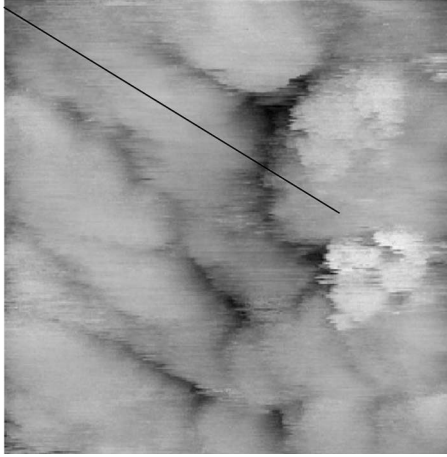
FIG. 22. STM image of 0.1% Br etched overdoped BSCCO ( T_C=74 K) at room temperature. Scan size is 800 \text{ \AA} \times 800 \text{ \AA} .
