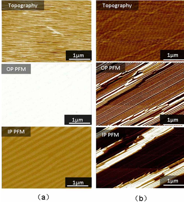
FIG. 2. (Color online) Large-area (5 \mu\text{m} \times 5 \mu\text{m} ) PFM images of (001) grown; (a) 71° and (b) 109° periodic domain structure.
