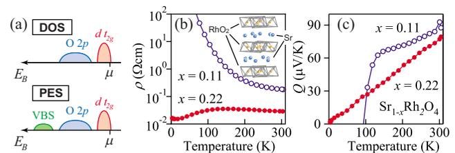
FIG. 1. (Color online)  $\text{Sr}_{1-x}\text{Rh}_2\text{O}_4$ , an analog of  $\text{Na}_{1-x}\text{CoO}_2$ . (a) Electronic structure. The band-theoretical DOSs of the cobaltates and the rhodates exhibit  $t_{2g}$  and O  $2p$  bands, but the valence-band PES spectra additionally exhibit VBSs. (b) Resistivity and (c) TE power of  $\text{Sr}_{1-x}\text{Rh}_2\text{O}_4$  as functions of temperature. The crystal structure of  $\text{SrRh}_2\text{O}_4$  is shown in the inset of (b).
