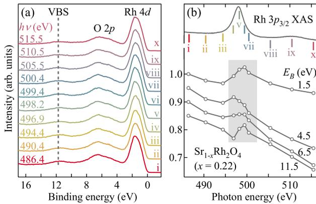
FIG. 2. (Color online) Rh  $3p$ - $4d$  resonant PES of  $\text{Sr}_{1-x}\text{Rh}_2\text{O}_4$  ( $x=0.22$ ). (a) Valence-band spectra recorded across the Rh  $3p_{3/2}$  edge. (b) CIS spectra and Rh  $3p_{3/2}$  XAS. CIS spectra are normalized to the intensity at 486.4 eV and have arbitrary offsets. The labels (i–x) on the spectra in (b) correspond to the photon energies indicated by bars on the Rh  $3p_{3/2}$  XAS in (c).
