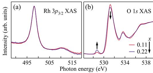
FIG. 4. (Color online) (a) Rh  $3p_{3/2}$  and (b) O  $1s$  XAS. The arrows in (b) indicate the change with increasing  $x$ .
