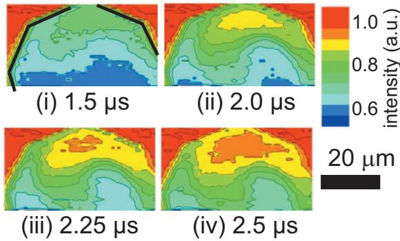
FIG. 2. (Color) X-ray microdiffraction images of a ferroelectric capacitor, acquired by forming maps of the intensity of the PZT 002 reflection. In images (i)–(iv) the polarization was partially switched by  $-1.43$  MV/cm electric field pulses of varying durations from a state initially poled in the opposite direction. The edge of the Pt top electrode is indicated by the line in image (i).
