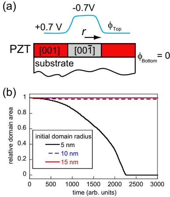
FIG. 5. (Color online) (a) Schematic of the electrostatic boundary conditions applied on the thin film to study the stability of cylindrical polarization domains using a phase-field model. (b) Fraction of the initial domain area remaining as a function of simulation time starting with cylindrical domains of several initial radii.
