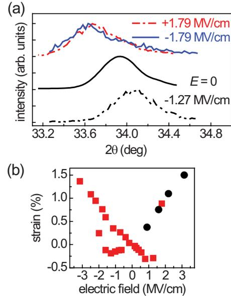
FIG. 1. (Color online). (a) Intensity vs  $2\theta$  angle for a  $\theta$ - $2\theta$  scan through the PZT 002 reflection for four magnitudes of 50 ns electric fields. (b) Piezoelectric strain for several electric fields, measured using 50 ns electric field pulses. The black circles are from Ref. 30.
