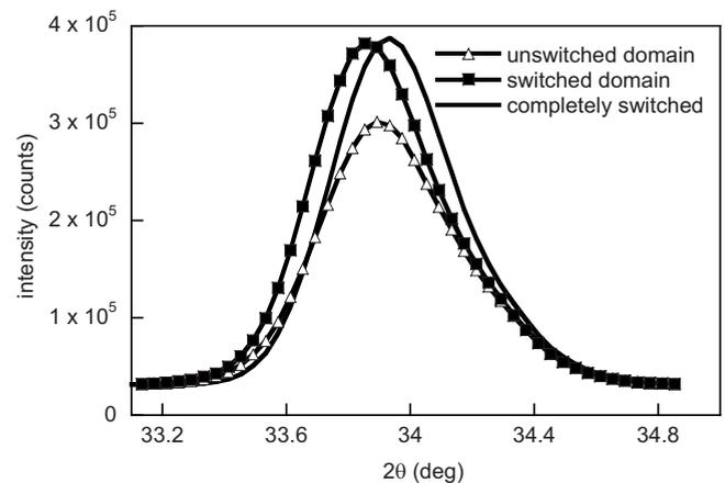
FIG. 4. Intensity vs  $2\theta$  angle in  $\theta$ - $2\theta$  scans at points within the switched and unswitched areas of image (ii) in Fig. 2 and after the switching has been completed. The difference in the integrated intensity of x-ray reflections is due to the difference between the structure factors of the PZT 002 and  $00\bar{2}$  reflections.
