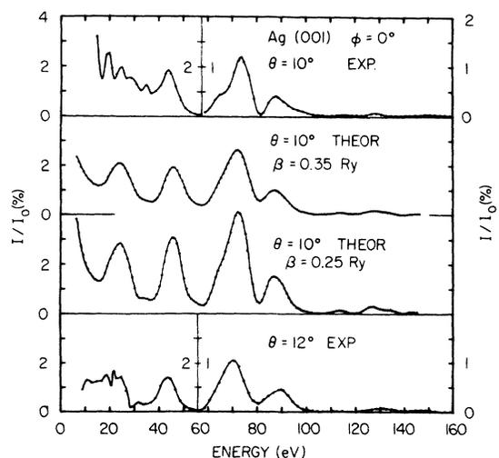
FIG. 6. LEED spectra from Ag{001}, 00 beam. Top: experimental ( $\theta = 10^\circ$ ,  $\phi = 0^\circ$ ). Middle: theoretical ( $\beta = 0.35$  Ry and  $\beta = 0.25$  Ry). Bottom: experimental ( $\theta = 12^\circ$ ,  $\phi = 0^\circ$ ).
