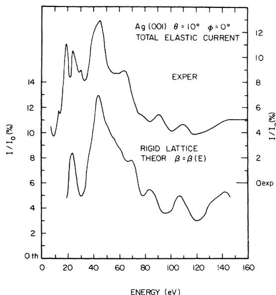
FIG. 8. Total elastic current reflected from Ag{001} at  $\theta=10^\circ$ ,  $\phi=0^\circ$ . Top curve: experimental. Bottom curve: theoretical (rigid lattice,  $\beta$  variable with energy as in Fig. 7).
