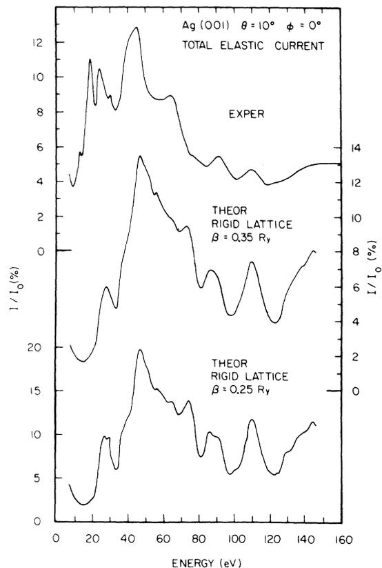
FIG. 2. Total elastic current reflected from Ag{001} at  $\theta=10^\circ$ ,  $\phi=0^\circ$ . Top curve: experimental. Middle curve: calculated (rigid lattice,  $\beta=0.35$  Ry). Bottom curve: calculated (rigid lattice,  $\beta=0.25$  Ry).
