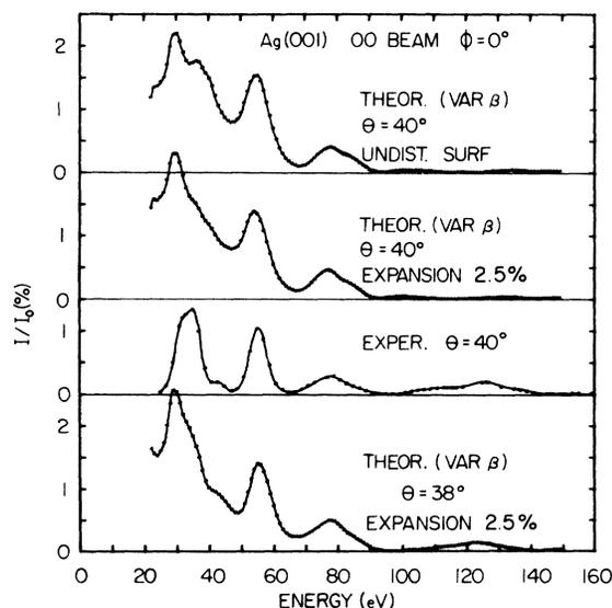
FIG. 14. LEED spectra from Ag{001}. Experimental curve (second from bottom) for  $\theta = 40^\circ$ , theoretical curves calculated for abrupt termination of the bulk (top) and for surface expanded by 2.5% (second from top) at  $\theta = 40^\circ$ , and for surface expanded by 2.5% at  $\theta = 38^\circ$  (bottom), all with variable  $\beta$ .
