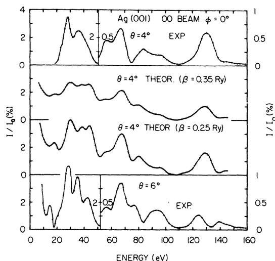
FIG. 5. LEED spectra from Ag{001}, 00 beam. Top: experimental ( $\theta = 4^\circ$ ,  $\phi = 0^\circ$ ). Middle: theoretical ( $\beta = 0.35$  Ry and  $\beta = 0.25$  Ry). Bottom: experimental ( $\theta = 6^\circ$ ,  $\phi = 0^\circ$ ).
