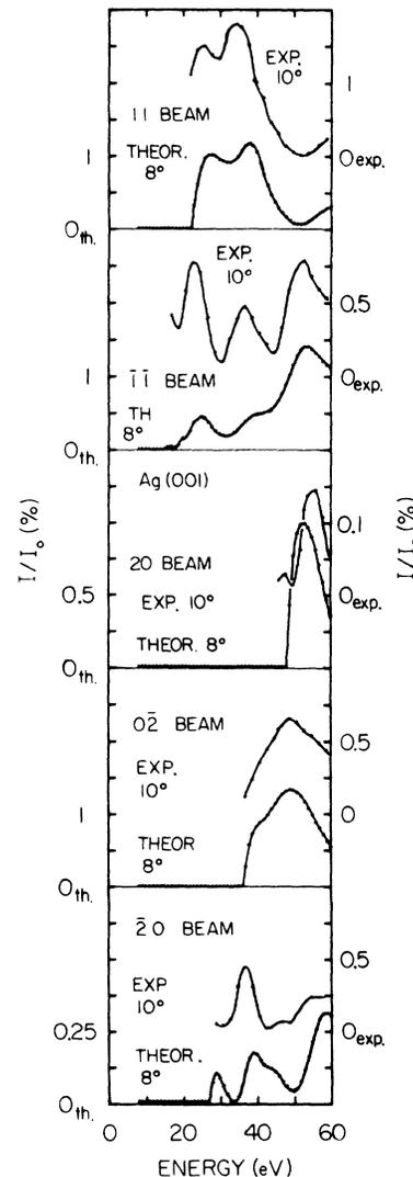
FIG. 12. Nonspecular LEED spectra in the energy range up to 60 eV from Ag{001} (compare with Fig. 9). Theoretical curves calculated for  $\theta = 8^\circ$ , experimental curves reported for  $\theta = 10^\circ$ .
