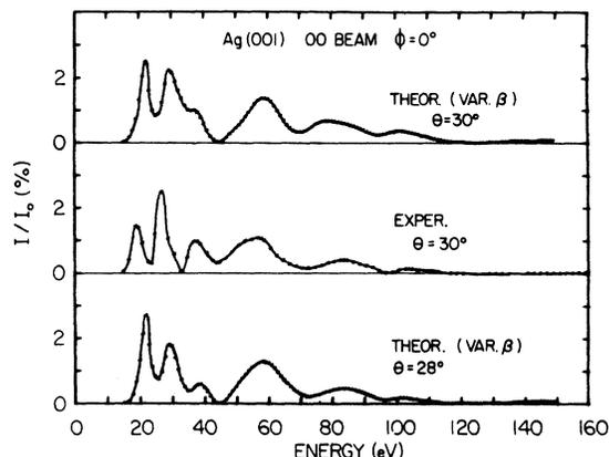
FIG. 13. LEED spectra from Ag{001}. Experimental curve (middle) for  $\theta = 30^\circ$ , theoretical curves (top and bottom) for  $\theta = 30^\circ$ , and  $\theta = 28^\circ$ , respectively, and variable  $\beta$ .
