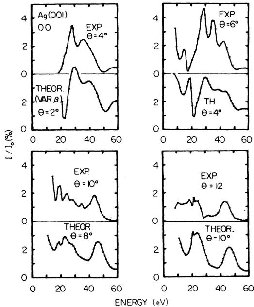
FIG. 11. LEED spectra from Ag{001} in the energy range up to 60 eV. The theoretical curves are all calculated for  $2^\circ$  less in  $\theta$  than the labeled values of  $\theta$  on the experimental curves.
