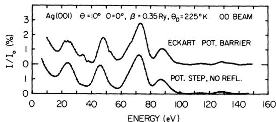
FIG. 10. Effect of surface potential barrier on LEED spectra of Ag{001}: 00 beam,  $\theta=10^\circ$ ,  $\phi=0^\circ$ .
