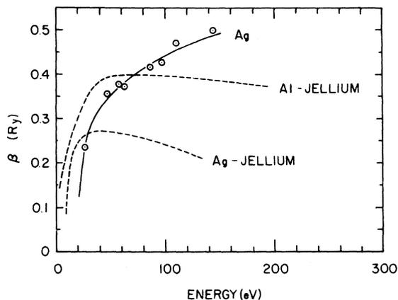
FIG. 7. Imaginary part  $\beta$  of the scattering potential as a function of electron energy. Solid curve: result of fitting procedure described in the text. Dashed curves: results obtained from Lundqvist calculations for jellium (Ref. 19) adapted to aluminum and silver.
