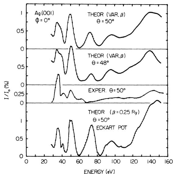
FIG. 15. LEED spectra from Ag{001}. Experimental curve (second from bottom) for  $\theta = 50^\circ$ , theoretical curves calculated with variable  $\beta$  for  $\theta = 50^\circ$  (top),  $\theta = 48^\circ$  (second from top), and with constant  $\beta = 0.25$  Ry, for  $\theta = 50^\circ$  and Eckart potential barrier (bottom).
