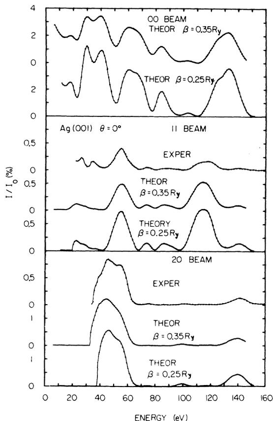
FIG. 4. LEED spectra from Ag{001} at normal incidence. Top panel: 00 beam, theoretical only ( $\beta = 0.35$  Ry and  $\beta = 0.25$  Ry). Middle panel: 11 beams, experimental and theoretical. Bottom panel: 20 beams, experimental and theoretical.
