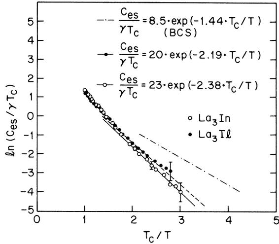
FIG. 3. Electronic specific heat in the superconducting state for  $\text{La}_3\text{In}$  and  $\text{La}_3\text{Tl}$ . Dash-dotted line, electronic specific heat as expected from BCS theory; full line and dotted line, fitted electronic specific heat at  $T_c/T > 2.5$  for  $\text{La}_3\text{In}$  and  $\text{La}_3\text{Tl}$ , respectively.
