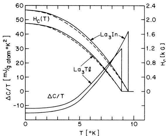
FIG. 4. Difference of measured specific heats in the superconducting and the normal state,  $\Delta C/T = (C_s - C_n)/T$ , and thermodynamical critical fields  $H_c(T)$  obtained from  $\Delta C/T$ . Dashed line,  $H_c^{\text{parab}} = H_c(0)[1 - (T/T_c)^2]$ .
