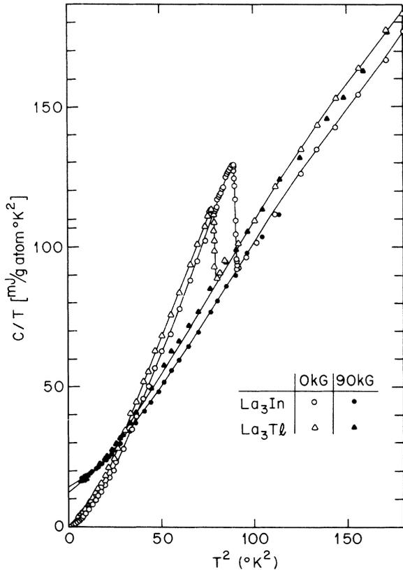
FIG. 1. Low-temperature specific heats for  $\text{La}_3\text{In}$  and  $\text{La}_3\text{Tl}$  in the normal and the superconducting state as measured in zero magnetic field and in a field of 90 kOe.
