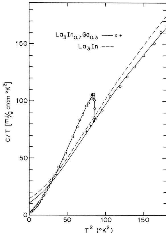
FIG. 6. Low-temperature specific heat for  $\text{La}_3\text{In}_{0.7}\text{Ga}_{0.3}$ .
