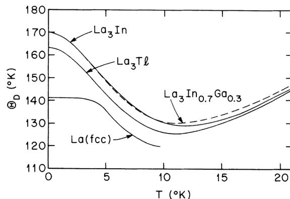
FIG. 2. Debye temperatures  $\Theta_D(T)$  as a function of temperature. For comparison,  $\Theta_D(T)$  of fcc La (from Ref. 3) is also reproduced.
