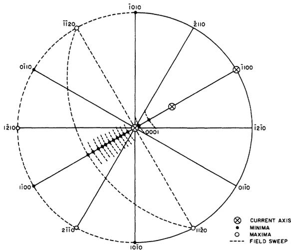
FIG. 9.  $\langle 0001 \rangle$  projection plot showing current axes and positions of maxima and minima observed in the transverse rotation curves of cobalt. Successive minima indicated in the  $(11\bar{2}0)$  plane were obtained by tipping the crystal with current  $40^\circ$  off *c* axis. The angular dependence of the Shubnikov-de Haas oscillations was measured using these successive field directions.
