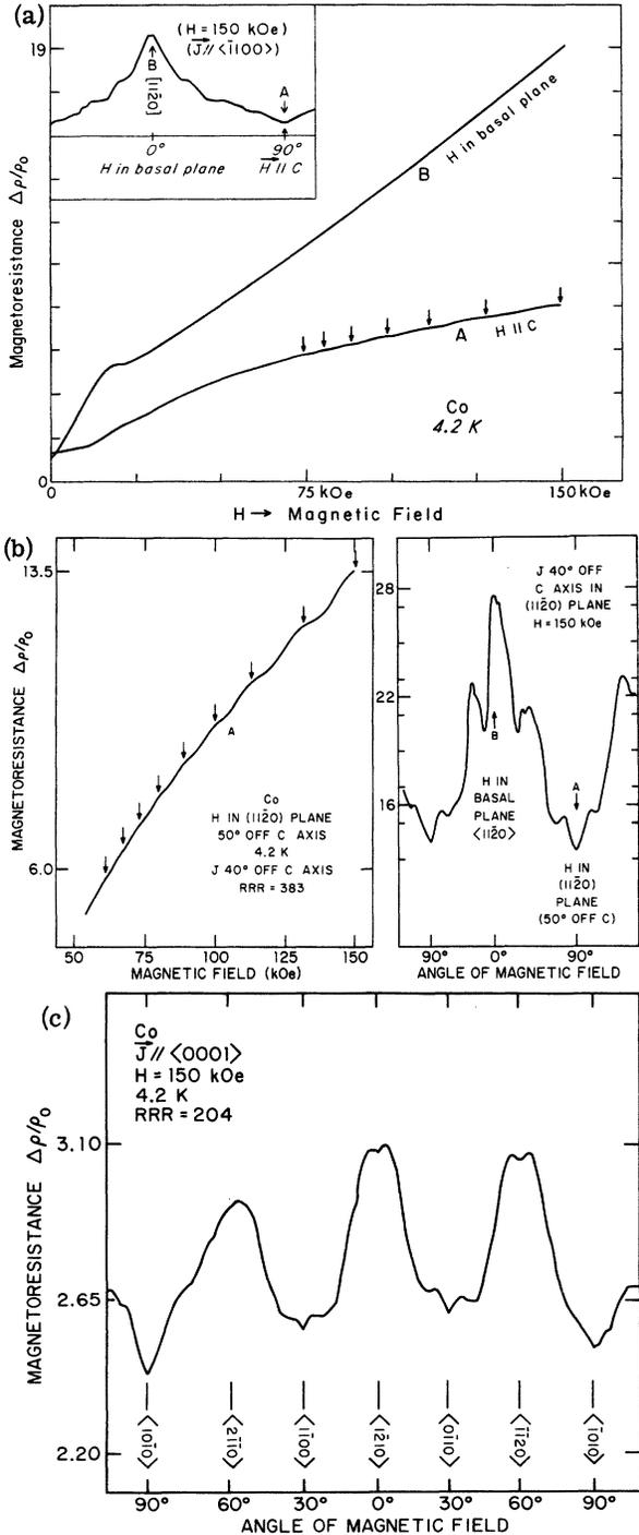
FIG. 8. Transverse magnetoresistance rotation diagrams and field sweeps for cobalt specimens. (a) Current in the basal plane parallel to a [110] direction. (b) Current in the (1120) plane 40° off the c axis. (c) Current parallel to the c axis.
