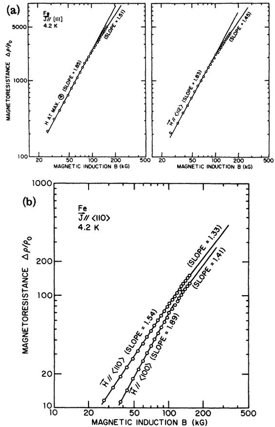
FIG. 6. Log-log plots of the relation  $\Delta\rho/\rho_0 = aB^n$  with values of  $n$  indicated by the slopes determined from the solid lines. (a)  $\langle 111 \rangle$  axial iron specimen in transverse orientation. Maximum at 4 (the circled 4) is indicated in Fig. 7(a). (b)  $\langle 110 \rangle$  axial iron specimen in transverse orientation.
