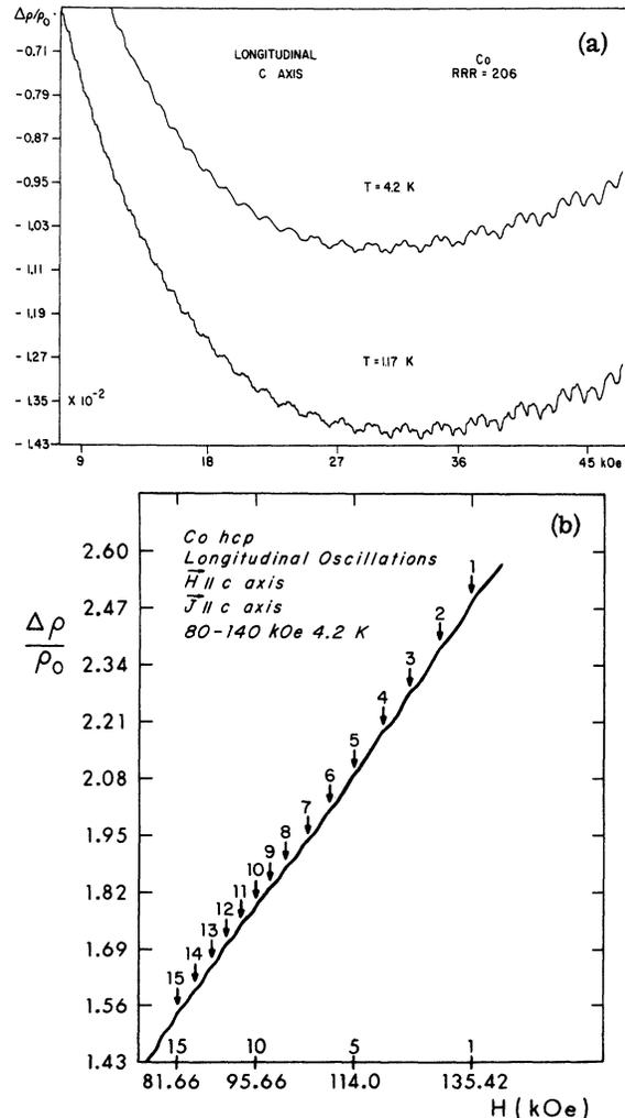
FIG. 11. Longitudinal Shubnikov-de Haas oscillations in cobalt observed with field and current along the *c* axis. (a) Oscillations in field range 0–50 kOe. (b) Oscillations in field range 80–140 kOe.
