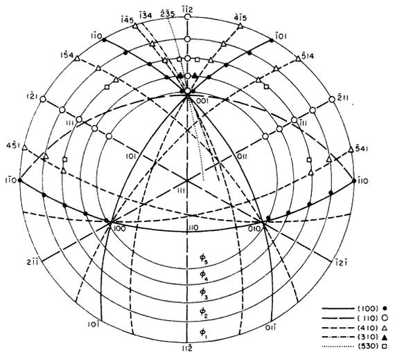
FIG. 5.  $\langle 111 \rangle$  projection plot showing field sweeps and positions of minima observed in the magnetoresistance-rotation curves for iron shown in Fig. 4. Relevant low-index planes are also indicated and coded as shown in lower right-hand side. The light solid curves labeled  $\phi_1$ ,  $\phi_2$ ,  $\phi_3$ ,  $\phi_4$ , and  $\phi_5$  represent the field sweeps. Data for  $\phi_2$ – $\phi_5$  are shown in Fig. 4.
