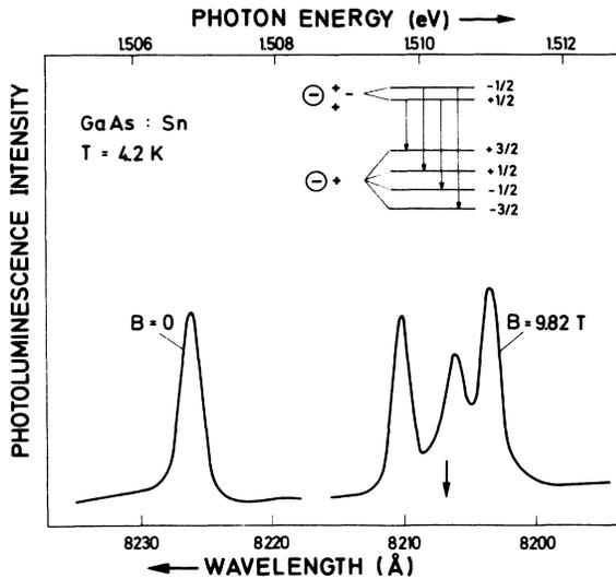
FIG. 1. Photoluminescence spectra of the bound-exciton line measured in the Faraday configuration. The Zeeman pattern is due to the splitting as shown by the term scheme. The arrow represents the center of gravity used to determine the ground-state energy shift.
