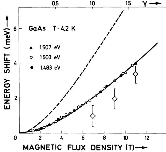
FIG. 2. Shift of the center of gravity for excitons bound to Sn ( $\Delta$ ) and Cu acceptors ( $\bullet$ ,  $\circ$ ). The solid line through the experimental points is calculated by Larsen's theory. The  $\gamma$  scale corresponds to the calculated mass  $\mu_{\text{expt}} = 0.068 m_e$ . The dashed line represents the calculated magnetic shift of an exciton with  $\mu_0 = 0.044 m_e$ .  $\diamond$  represents the magnetic shift of the free exciton measured in absorption after Ref. 10.
