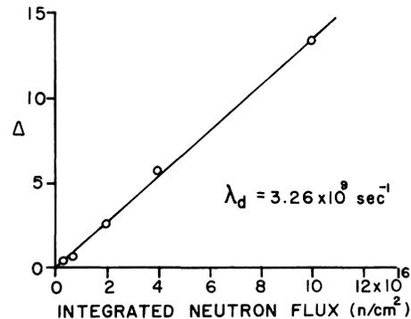
FIG. 3. Value of  $\Delta$  vs integrated neutron flux.
