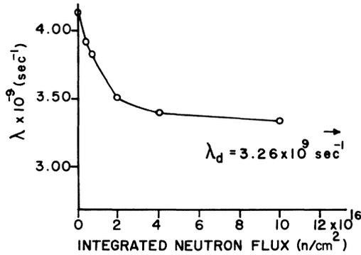
FIG. 2. Annihilation rate vs integrated neutron flux.
