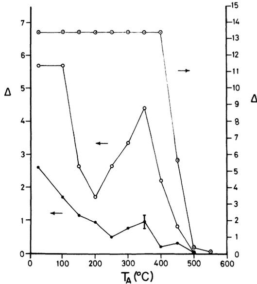
FIG. 4. Isochronal-annealing data from three pairs of samples irradiated with  $2 \times 10^{16}$  (darkened circle),  $4 \times 10^{16}$  (open circle), and  $1 \times 10^{17}$  fast neutrons/cm<sup>2</sup> (circle with a dot).
