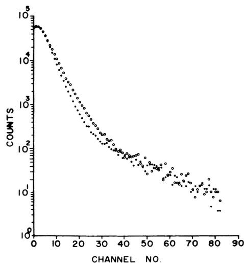
FIG. 1. Typical delay-time spectra between 1.28-MeV  $\gamma$  rays and 0.51-MeV positron-annihilation rays from a pair of  $100$ - $\Omega$  cm *p*-type silicon samples before and after an irradiation of  $1\times 10^{17}$  fast neutrons/cm<sup>2</sup>.
