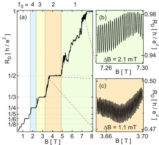
FIG. 2. (Color online) Oscillations in  $R_D$  as a function of magnetic field  $B$  for the  $2.0 \mu\text{m}^2$  device. (a)  $R_D$  as a function of  $B$ , showing well-quantized integer plateaus. Different colored backgrounds indicate different numbers of fully occupied LLs ( $f_0$ ) through the device. [(b) and (c)] Zoom ins of the data in (a), at  $f_0 = 1$  and  $2$ , respectively, showing oscillations in  $R_D$ , and their  $B$  periods  $\Delta B$ .
