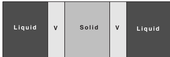
FIG. 1. Conceptual representation of the experiment showing the sandwich-like geometry with three chambers, each pair of which is separated by a region of liquid helium-filled porous Vycor glass, V. In operation a temperature difference is applied across each of the regions of Vycor, which keeps the liquid reservoirs from freezing.
