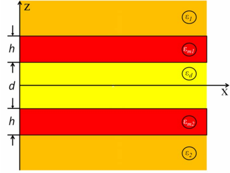
FIG. 1. (Color online) Geometry of a five-layer system formed by a dielectric film (thickness d , permittivity \epsilon_d ) sandwiched between two metal layers (thickness h , permittivity \epsilon_{m1} and \epsilon_{m2} ) and surrounded by two semi-infinite dielectric layers (permittivities \epsilon_1 and \epsilon_2 ).
